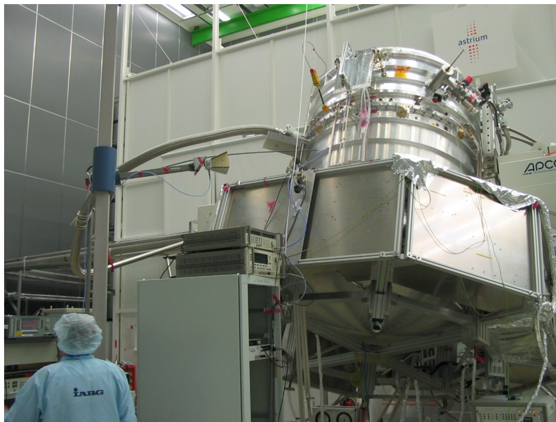
Fig. 8.2-3: Antenna Lower Position for HIFI Biasing Harness
