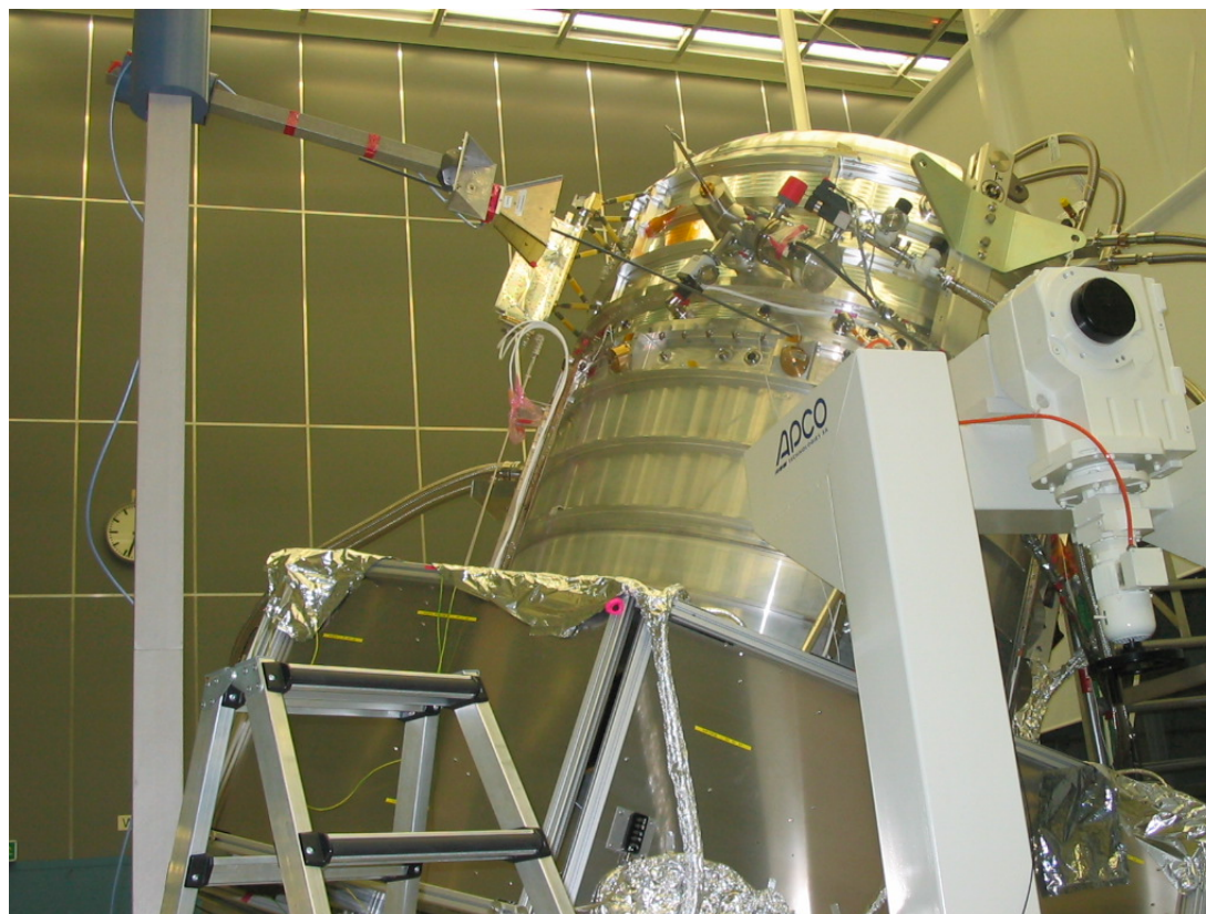
Fig. 8.8-4: Second Antenna Position for the SPIRE E-field RS Test, 1 GHz to 18 GHz
