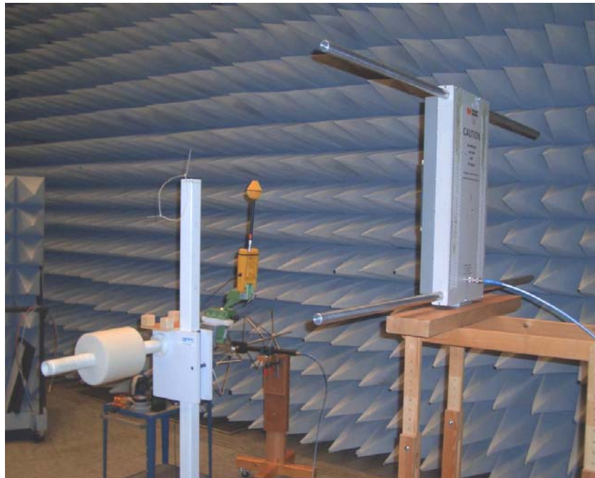
FIG 3: Calibration Setup 14 kHz – 30 MHz with AT-3000
