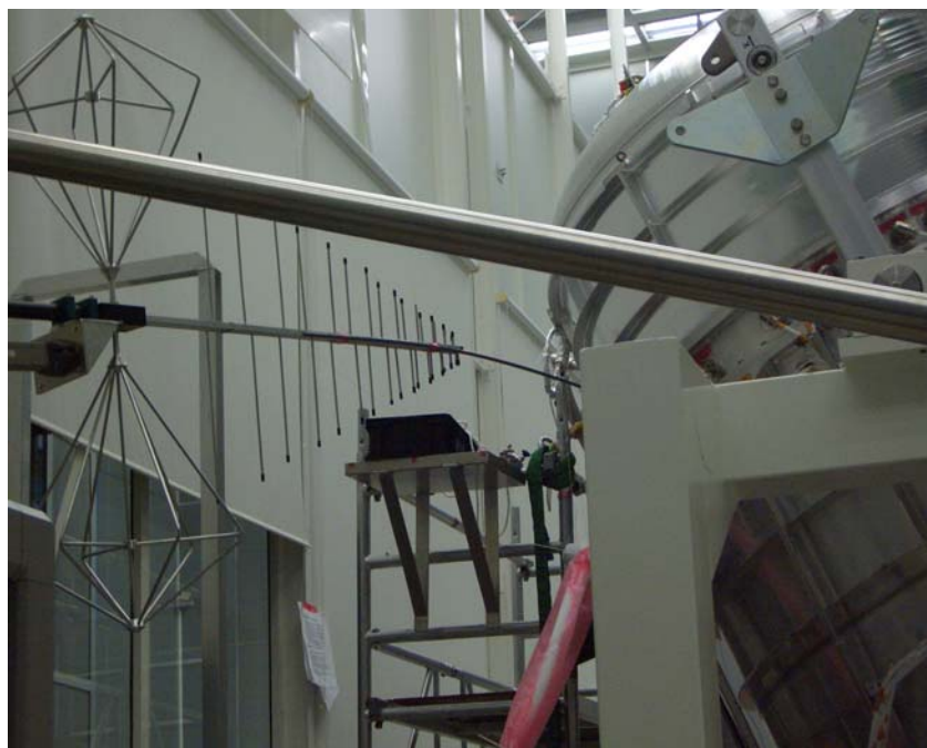
FIG 34: Setup RS E-Field 30 MHz – 1 GHz vertical on PACS in position 1
