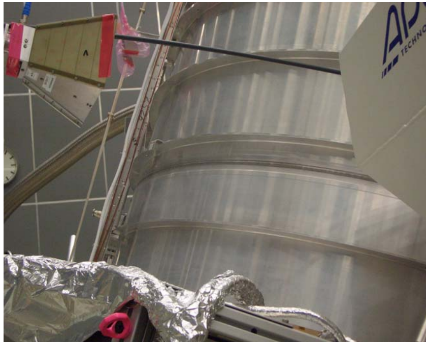
FIG 43: Setup RS E-Field 1 GHz -6 GHz vertical on SPIRE in position 1
