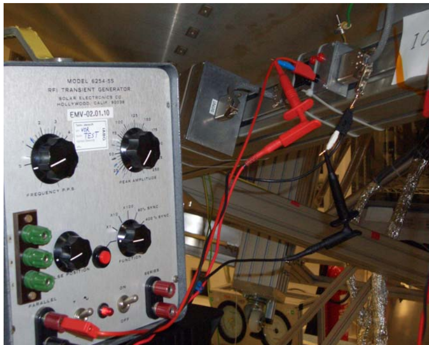
FIG 22: Test Setup for 10 \mu sec Transient
