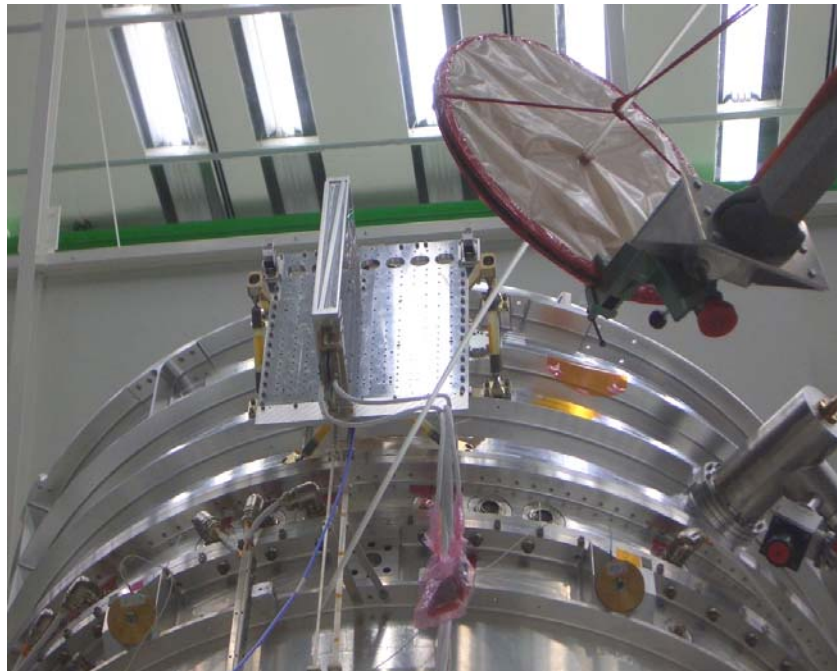
FIG 13: Setup RS H-Field on HIFI front view
