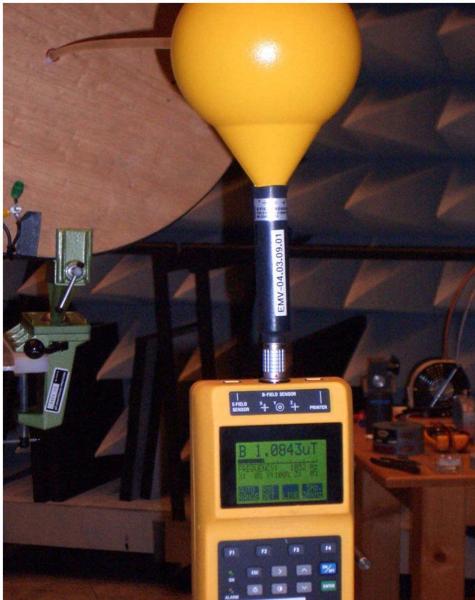
FIG 1: Calibration of Magnetic Field in IABG Anechoic Chamber
