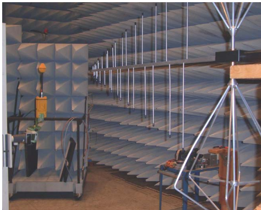
FIG 4: Calibration Setup 30 MHz – 1 GHz with BDLP vertical
