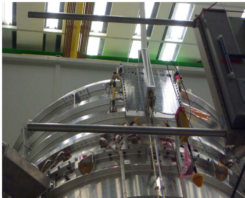
FIG 15: Setup RS E-Field 14 kHz – 30 MHz on HIFI in upper position
