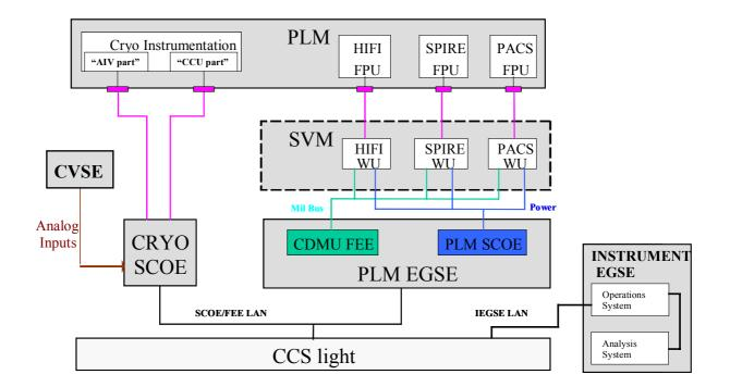
Figure 4-1: Principle Test Set-up for EQM Tests
