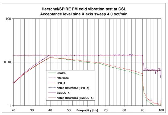
Figure 8.4-1 Achieved inputs for the X direction
