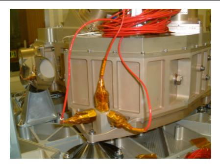
A-1: The triax on the photometer detector box
