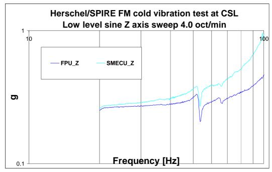
Figure 8.4-6 FPU\_Z and SMECU\_Z response (low level)
