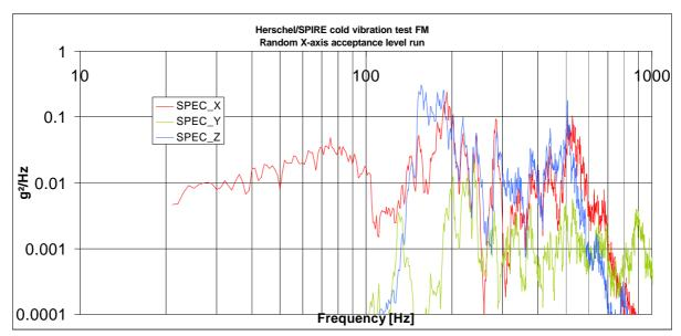
Figure 8.5-5 Achieved random input for spectrometer detector box
