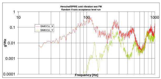
Figure 8.5-7 Achieved random input for the top of the spectrometer mechanism
