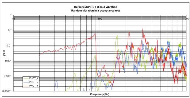
Figure 8.5-12 Y-axis response graph for photometer detector box
