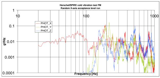
Figure 8.5-6 Achieved random input for photometer detector box
