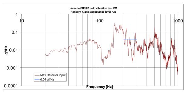
Figure 8.5-8 Maximum random input for (envelope) for the detectors
