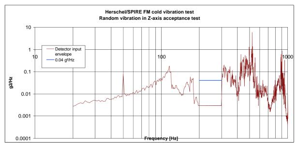
Table 8.5-20 Z-axis achieved detector input levels, too deeply notched between 200 ad 300 Hz
