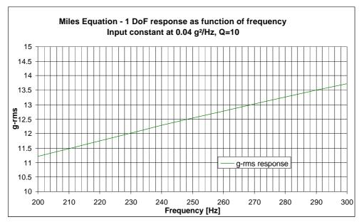
Figure 8.5-3: Miles response (as a function of frequency)
