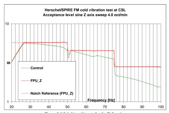
Figure 8.4-8 Achieved inputs for the Z direction
