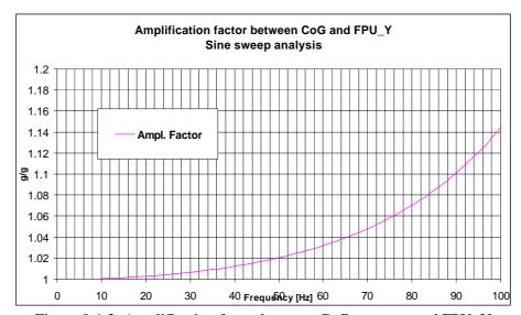
Figure 8.4-3: Amplification factor between CoG response and FPU\_Y
