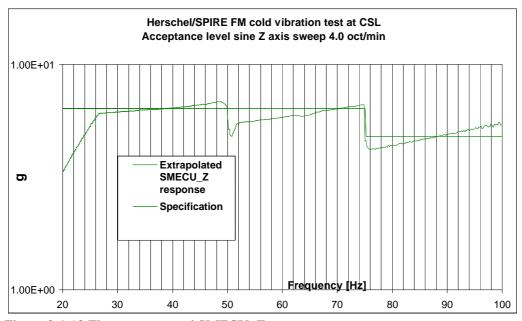
Figure 8.4-10 The reconstructed SMECU\_Z response
