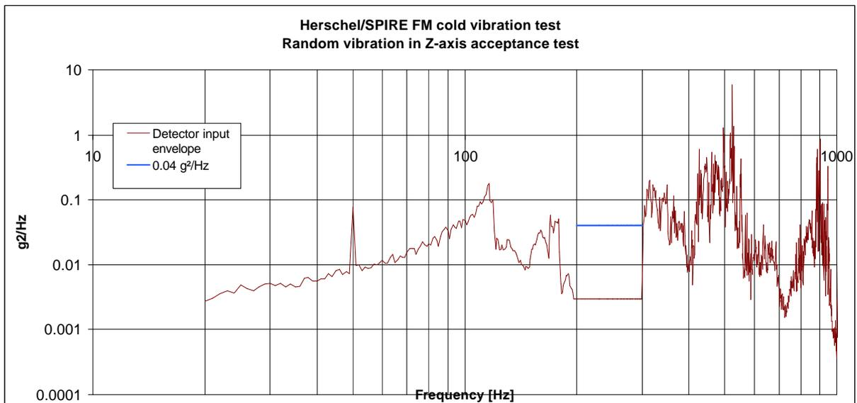
Table 8.5-20 Z-axis achieved detector input levels, too deeply notched between 200 and 300 Hz
