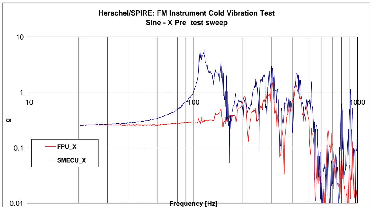
Figure 8.5-2: Filtered low level sine sweep response, note the (jagged) response of the SMEC between 110 and 120 Hz.
