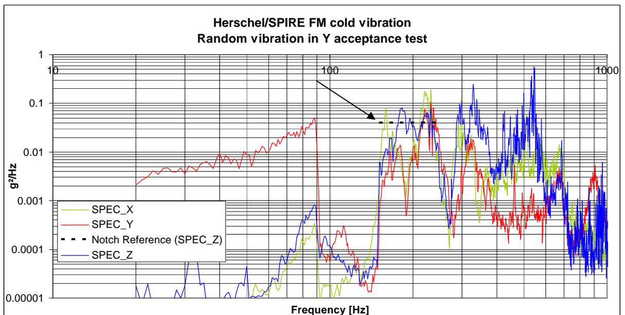
Figure 8.5-11 Y-axis response graph for spectrometer detector box, arrow points to notch level
