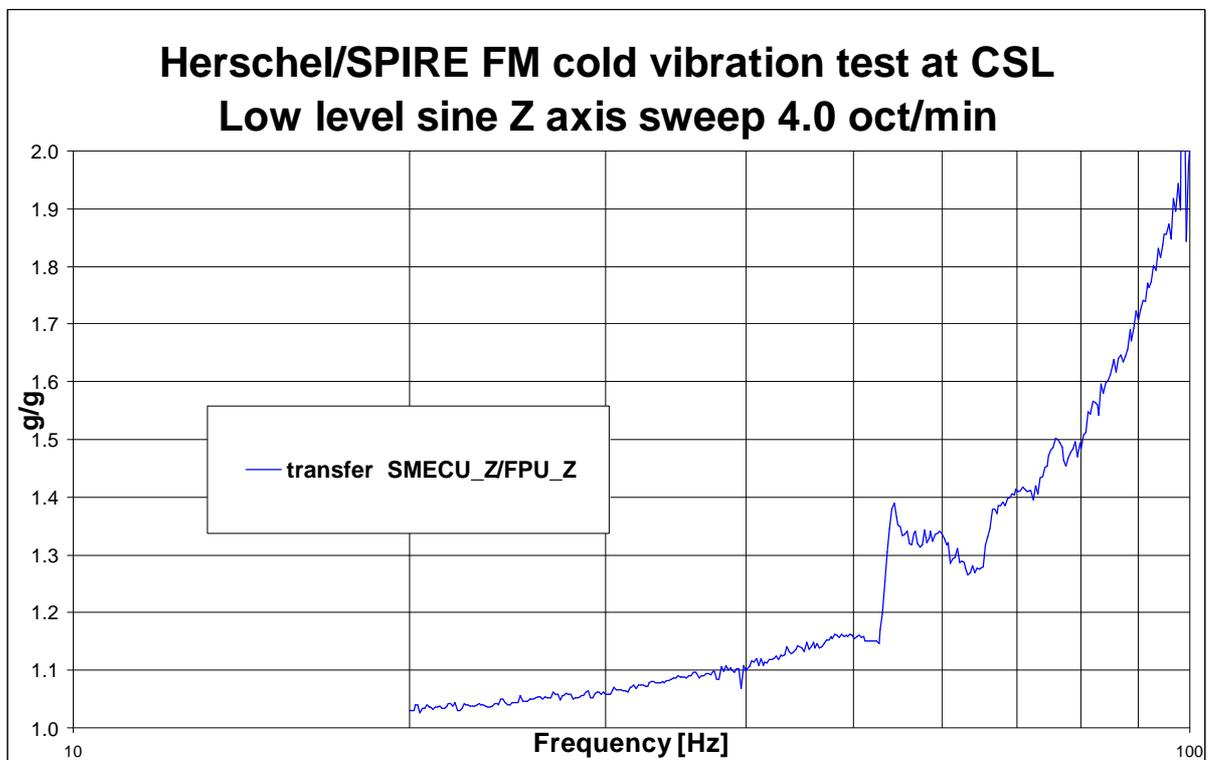
Figure 8.4-7 FPU\_Z and SMECU\_Z transfer function (low level)
