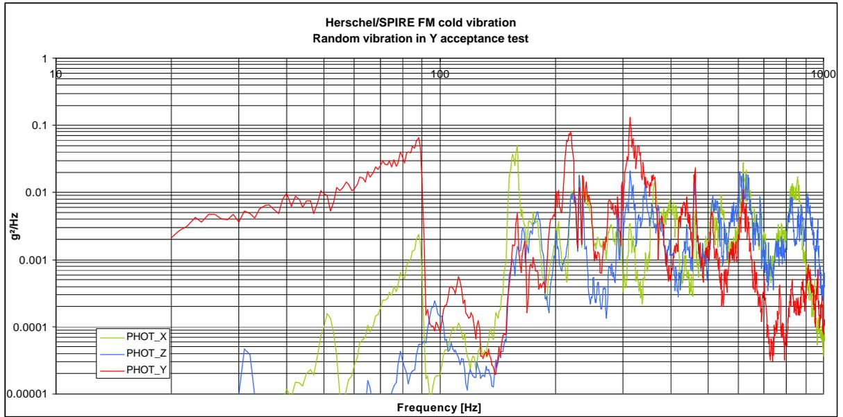
Figure 8.5-12 Y-axis response graph for photometer detector box
