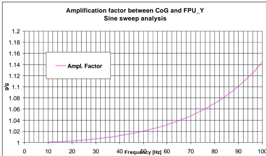
Figure 8.4-3: Amplification factor between CoG response and FPU\_Y
