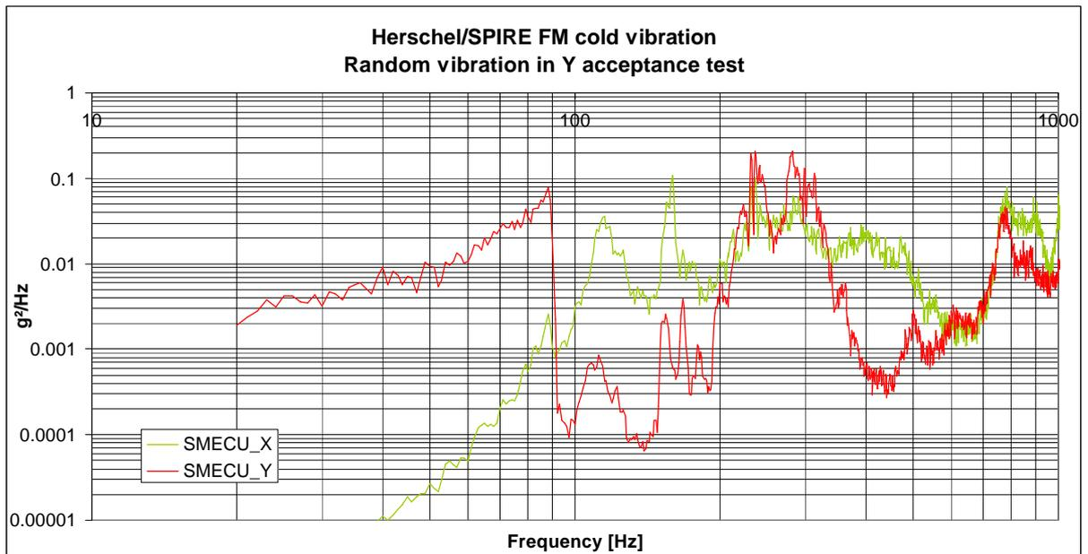
Figure 8.5-13 Achieved random input for the top of the spectrometer mechanism
