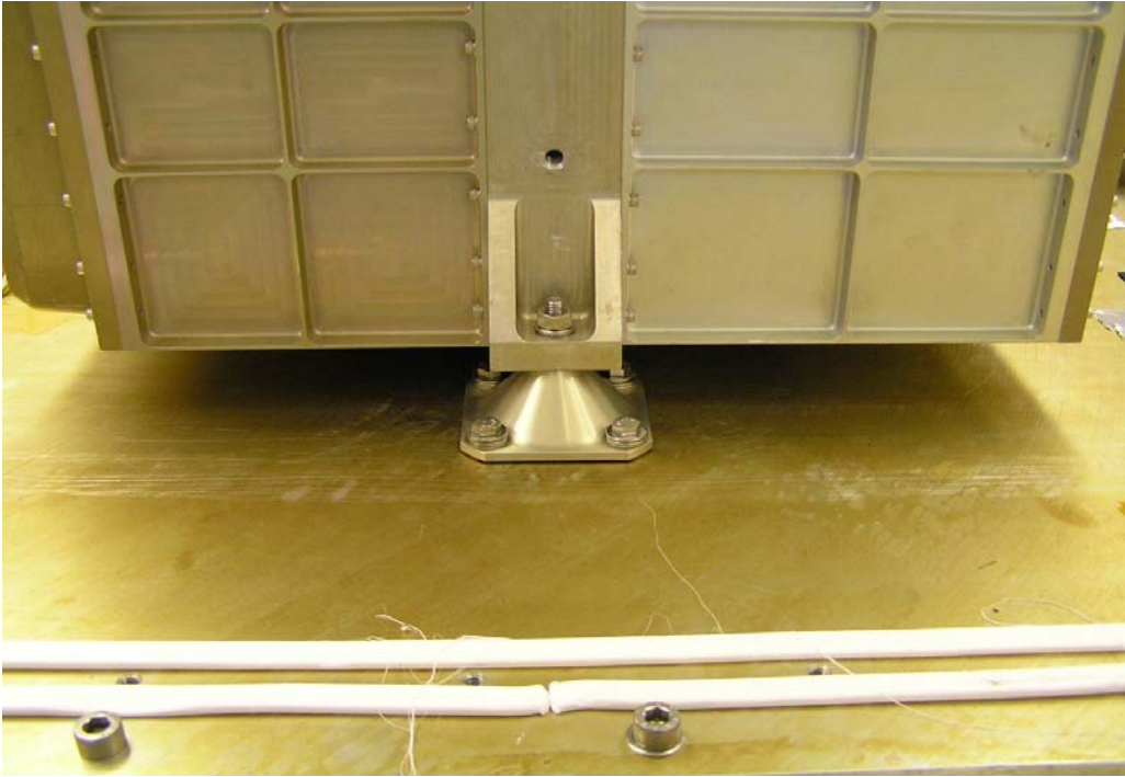
Transit Cone fitted
