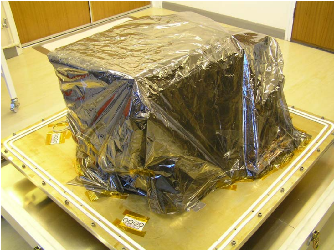
Metal Cover removed showing FPU double Bagged
