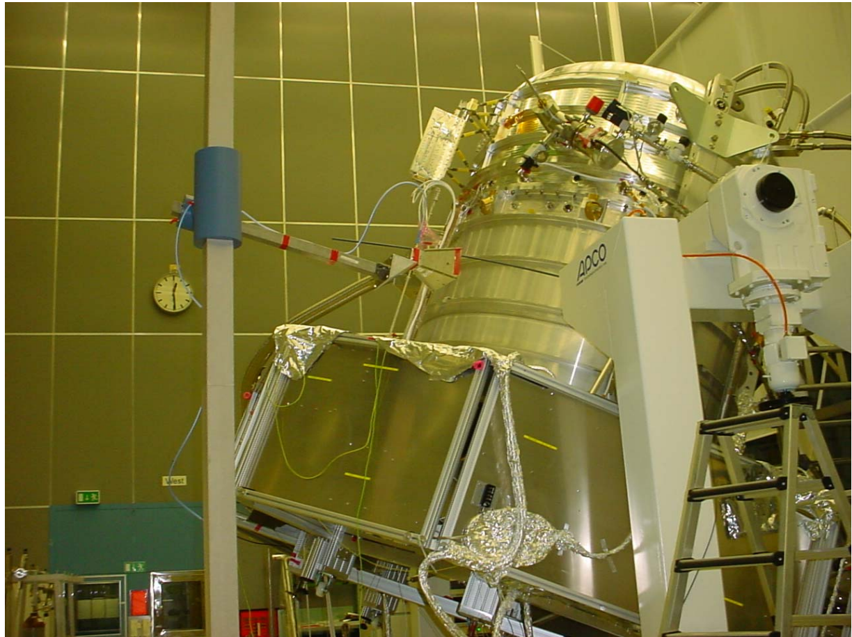
Figure 32 – Antenna location position 1, Vertical polarisation, 1-18GHz (1869.jpg)
