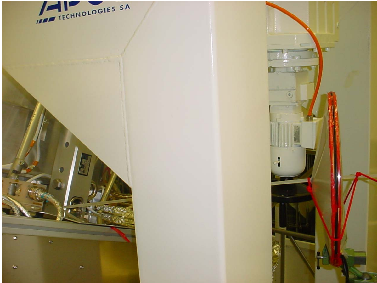
Figure 22 - View of Loop antenna for H-Field tests. The antenna is behind the cryostat dolly and the antenna is ~ 1m from the SPIRE SVM-CB (1838.jpg)
