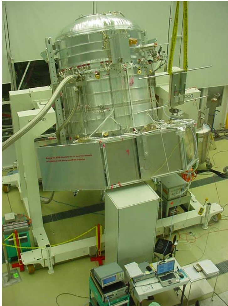
Figure 31 - Antenna Location #1 for E-Field 14kHz-30MHz Horizontal polarization. (1865.jpg)
