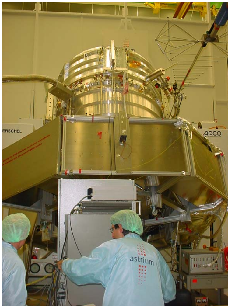
Figure 27 - Antenna Location #1 for E-Field 30MHz-1GHz Horizontal polarization. (1845.jpg)
