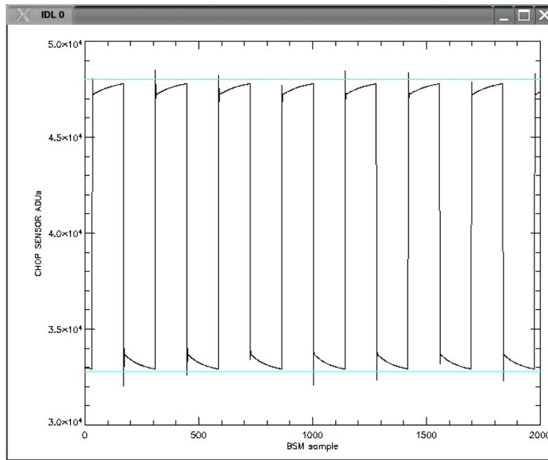
Here the previous feed forward gain we do not event reach the target position and the integral effect is dragging the mechanism to reach the desired position. Therefore a change in FFGAIN is required.
