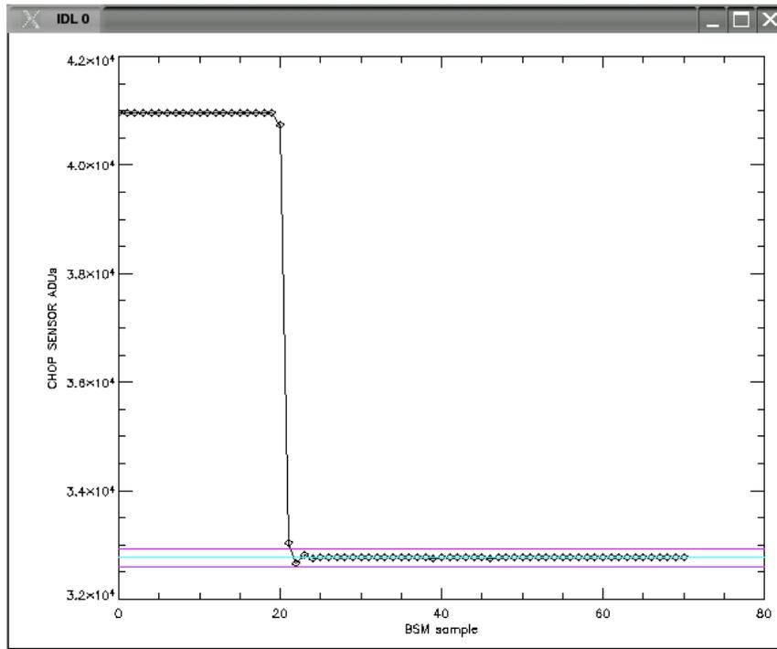
This figure shows the chop magneto resistive sensor signal on a 'step down' where the target position is shown in cyan and a 1 arcsec band is also included to check the settling time. The BSM samples
