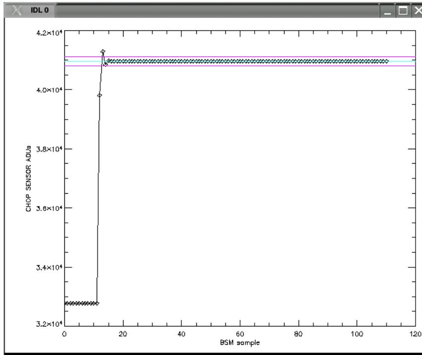
This figure shows the chop magneto resistive sensor signal on a 'step up' where the target position is shown in cyan and a 1 arcsec band is also included to check the settling time. The BSM samples (diamonds) are 8 ms apart (125 Hz BSM sampling).
