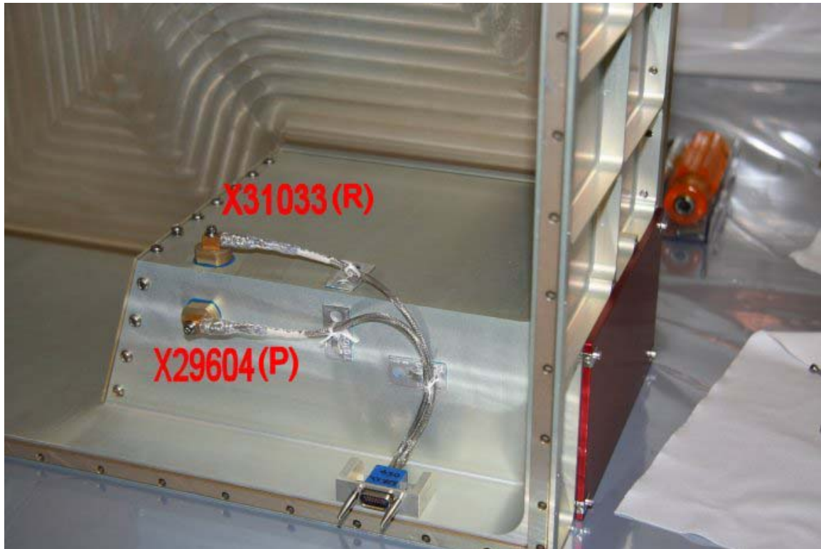
Figure 7-3 - HSFPU Input Baffle Flight Temperature Sensors
