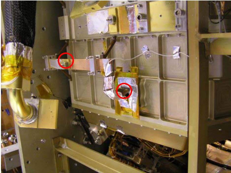
Figure 7-7 – L0 Detector Enclosure MGSE Strap Temperature Sensors
