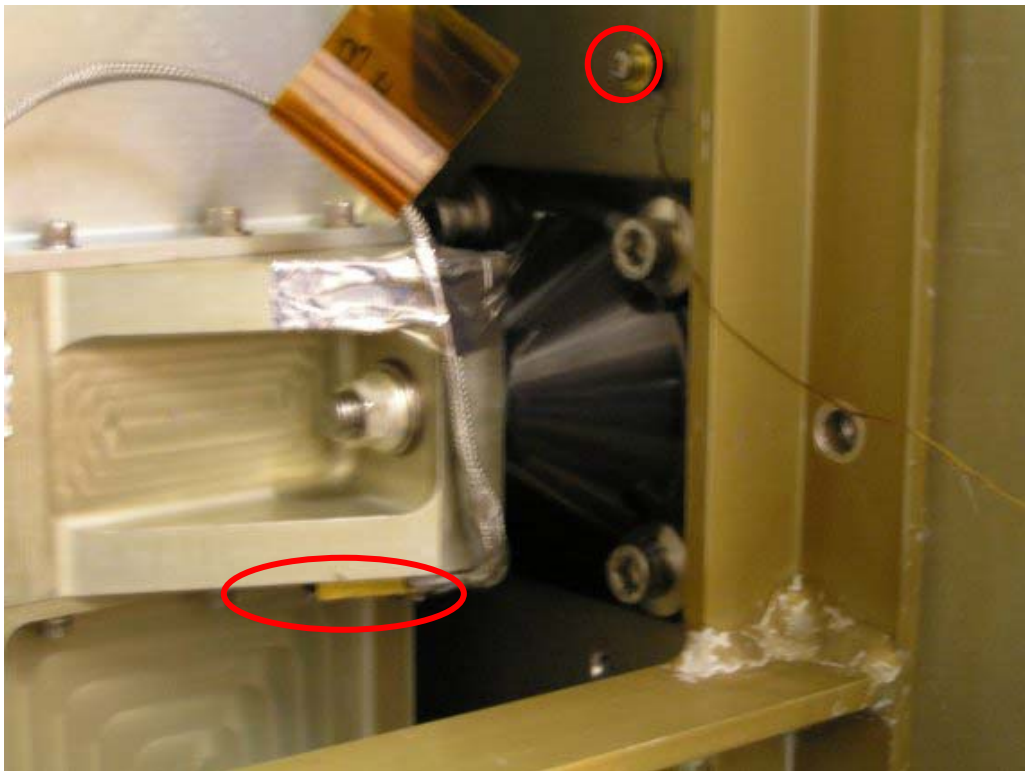
Figure 7-13 – L1 Cone Support Temperature Sensors
