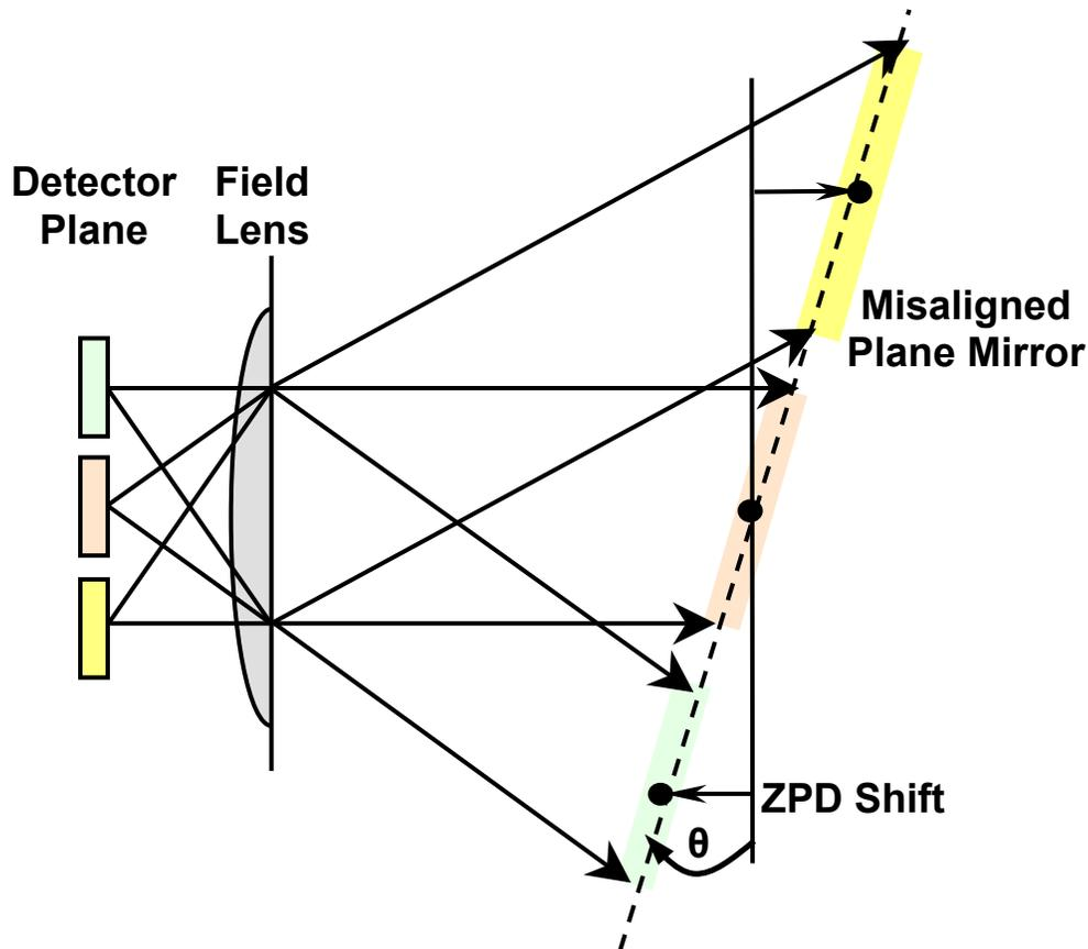
**Figure 6: Possible effects of a spectrometer misalignment.** The shaded areas correspond to the projection of the detector onto a plane mirror. The black circles represent the shifted ZPD positions for each of the detector pixels shown. (Figure not drawn to scale, misalignment exaggerated for clarity).
