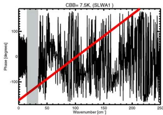
**Figure 2: Sample phase spectrum.** The phase spectrum shown here is derived from the sample interferogram above. The fit to the in-band phase is shown as the red line. The grey area corresponds to the SLW pass band.
