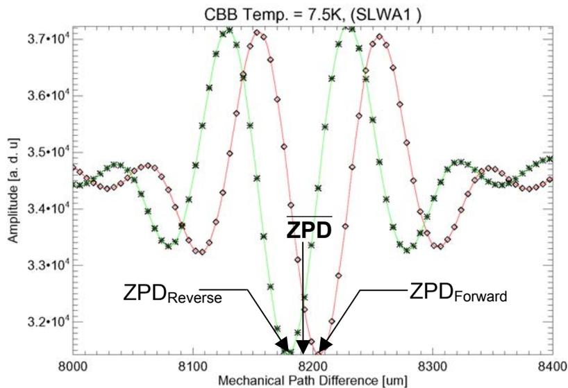
**Figure 4: Sample forward (\*) and reverse (◇) scans.** The solid lines show the result of the interpolation step (red: forward, green: reverse). Also indicated are the derived ZPD positions for each scan and the average ZPD position.
