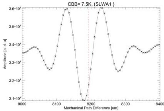
**Figure 1: Sample interferogram, initial guess at ZPD.** The dashed line shown denotes the initial guess at the ZPD position.
