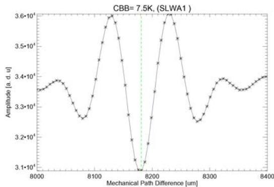
**Figure 3: Sample interferogram, corrected ZPD.** The dashed line shown here denotes the ZPD position derived from the initial guess and the linear fit to the resultant phase.
