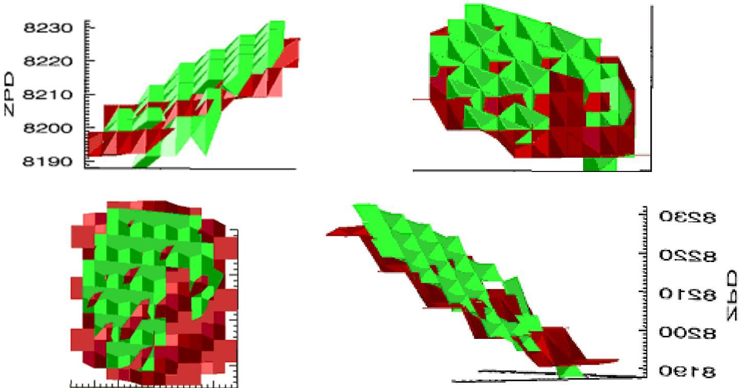
Figure 5: Surface plots of the distribution of the ZPD position. The plots shown are four different views of the distribution of derived ZPD positions (units: SMEC mirror position in  $\mu\text{m}$ ) across the **SLW** and **SSW** arrays for the data set where the CBB was set to 7.5K.
