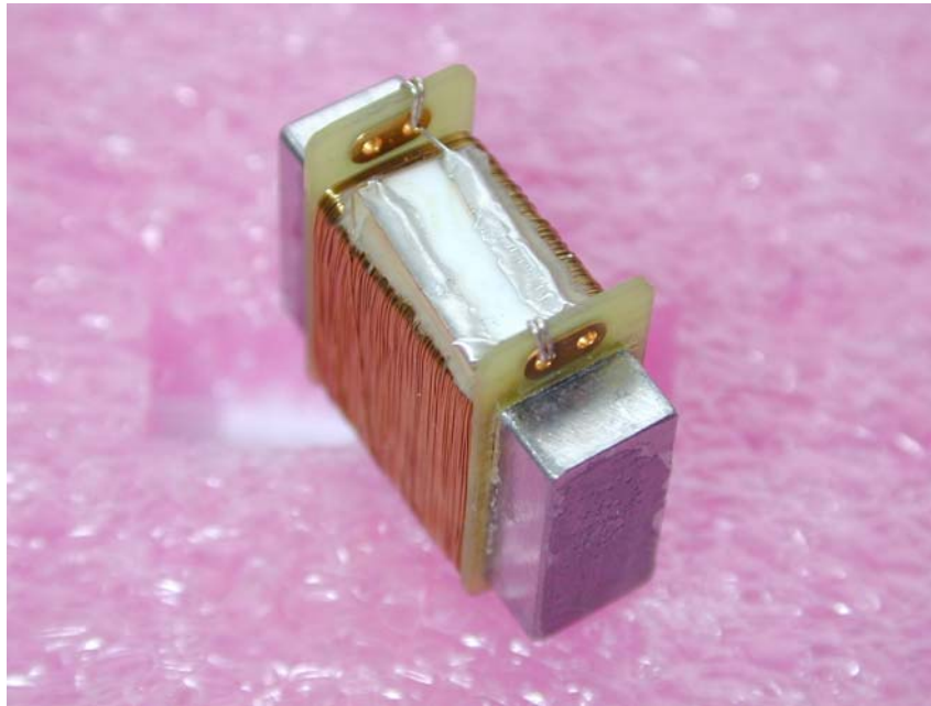
Figure 4-39 - Prototype BSM motor.
