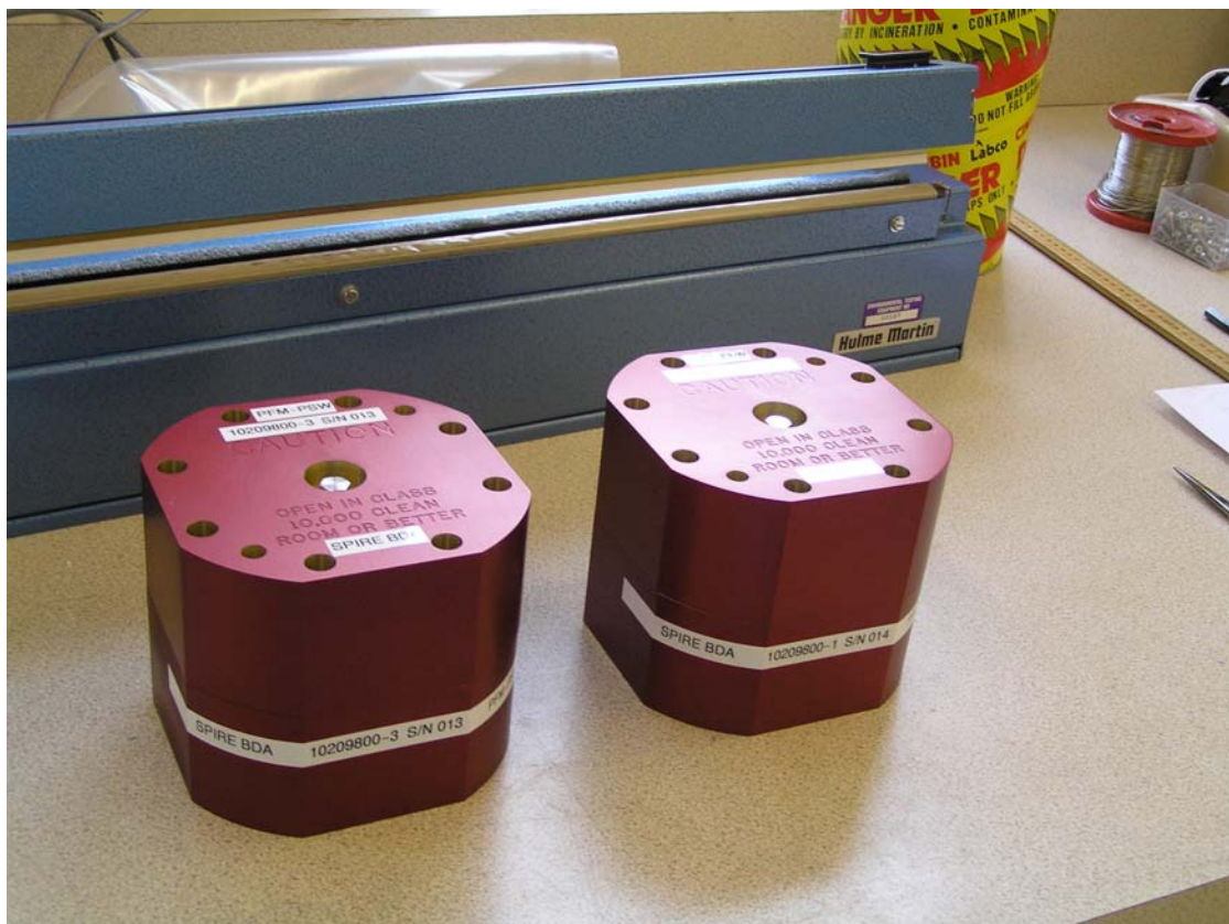
PFM BDA SN 13 & 14: In G56 Prep Area. Outside surfaces have been cleaned with IPA prior to taking into the Class 100 Clean Room for further inspection.
