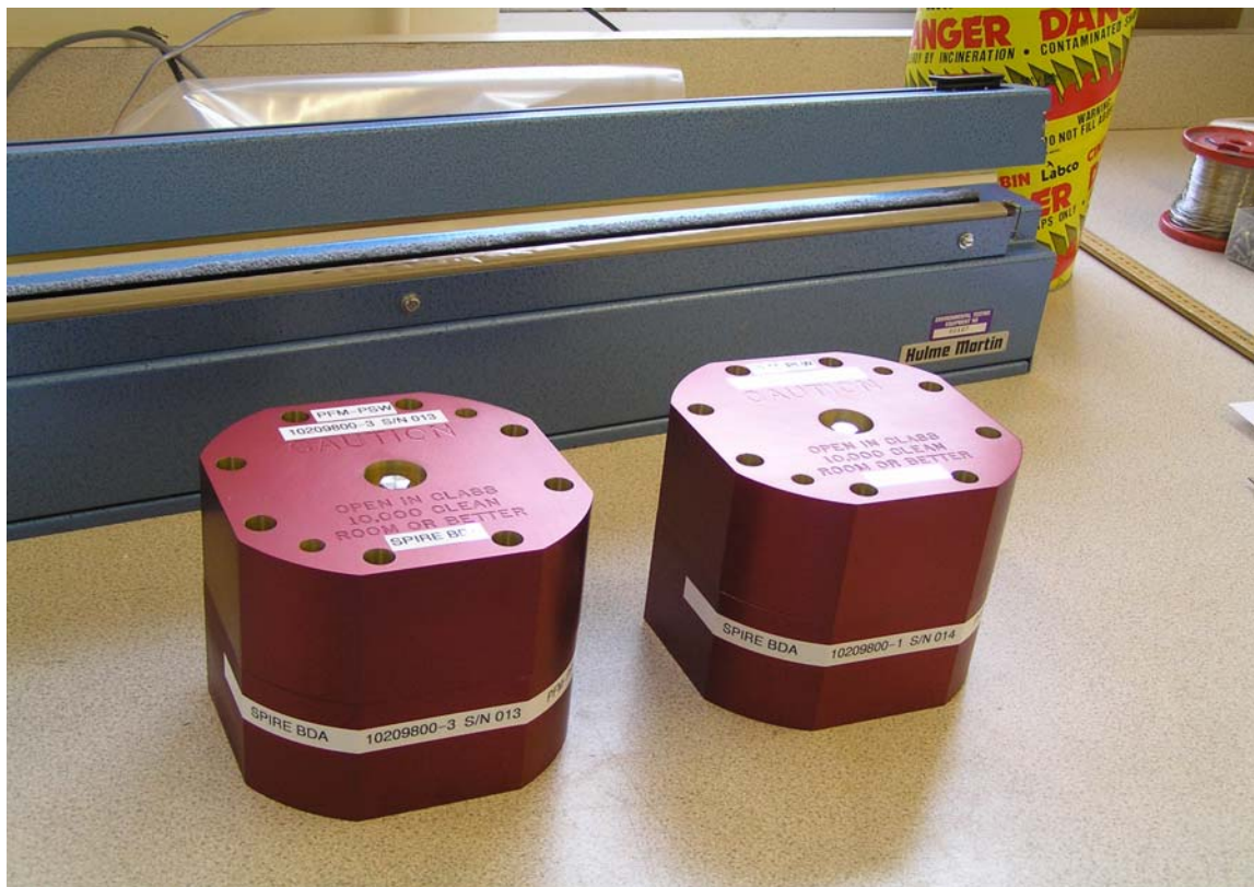
PFM BDA SN 13 & 14: In G56 Prep Area. Outside surfaces have been cleaned with IPA prior to taking into the Class 100 Clean Room for further inspection.
