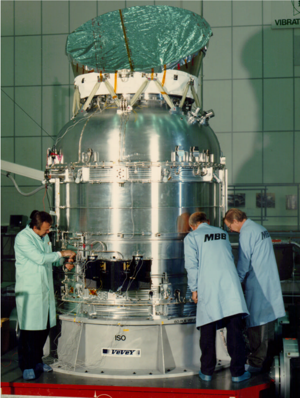
Figure 5-3: Preparation of the ISO PLM for the Vibration Test at IABG
