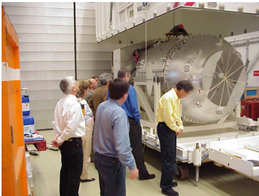
Figure 5-5: ISO PLM in the opened Transport Container at ESTEC
