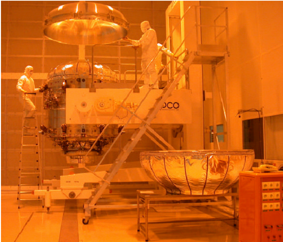
Figure 11-1: Herschel EQM in the class 100 cleanroom at ASTRIUM Ottobrunn, 5.6.02
