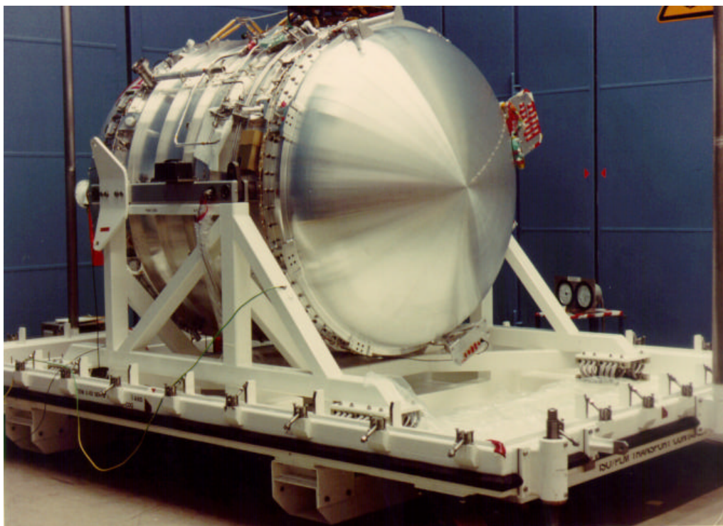
Figure 5-4: ISO PLM mounted in the Transport Container
