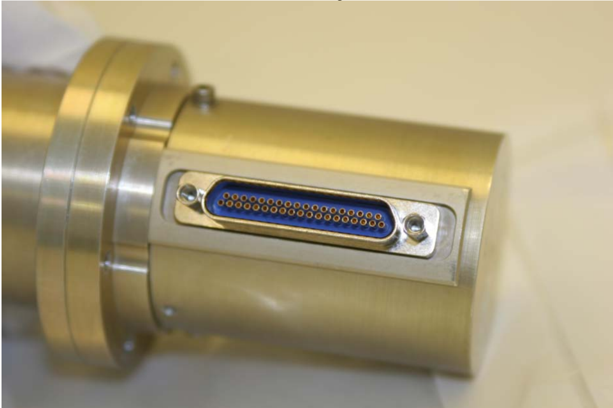
Photo 3 & 4 Prime & Redundant Connector Pin Alignment OK
