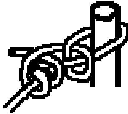
Figure 34 Details of knot used for terminating the Kevlar at capstans (Adjustable Jam Hitch).
