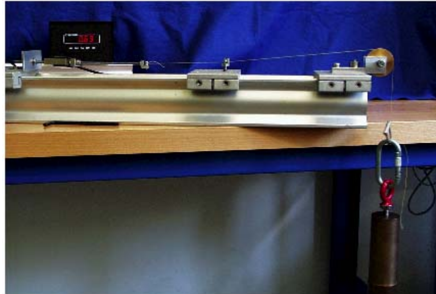
Figure 31 Experimental arrangement for capstan tests.
