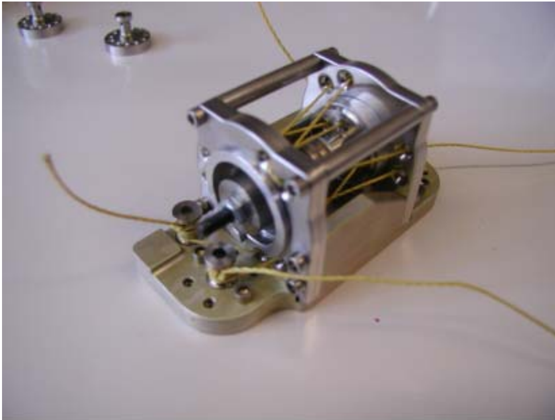
Figure 66 Assembled hub prior to hub compression release
