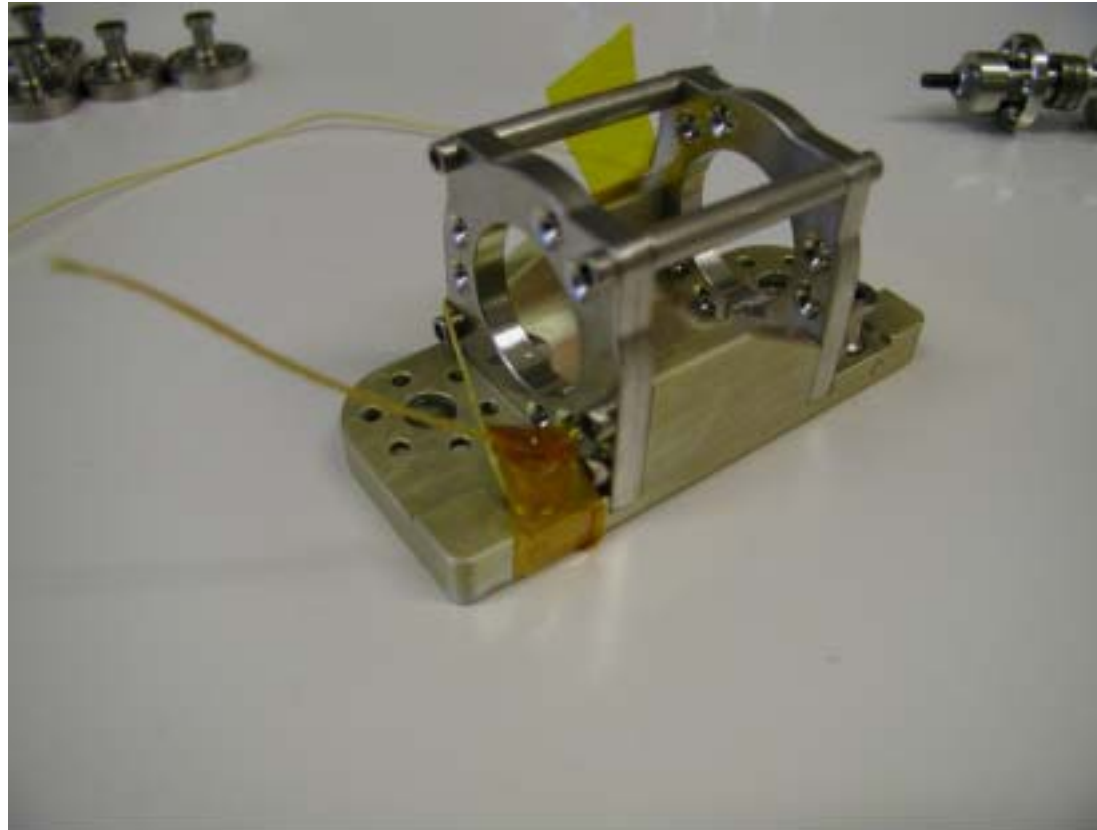
Figure 59 Kevlar tied and wrapped around fixed capstan, temporarily held with Kapton tape.
