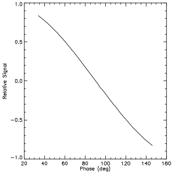
Figure 3: Relative signal as a function of phase between sine signal and square wave reference.
