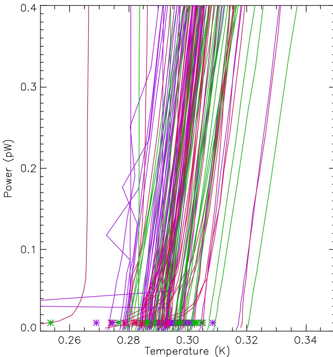
Figure 10: As figure 9 but close up of low power part of curve. Also plotted are temperatures found from the low bias part of the load curve a la Jamie. There is reasonable but not detailed agreement between the values. Also note that some of the 190 Hz curves have not been fully corrected by this method – the reason for this is not clear but probably associated with those channels where the out of phase data went negative.
