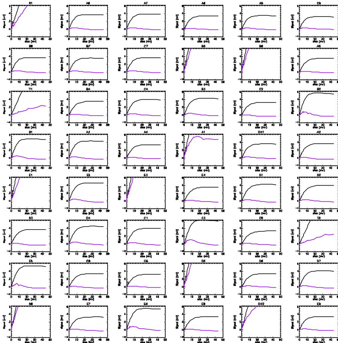
Figure 1: Comparison of dark load curves at 130 Hz with “peaked” phase (black) and 90 deg from peak (purple)
