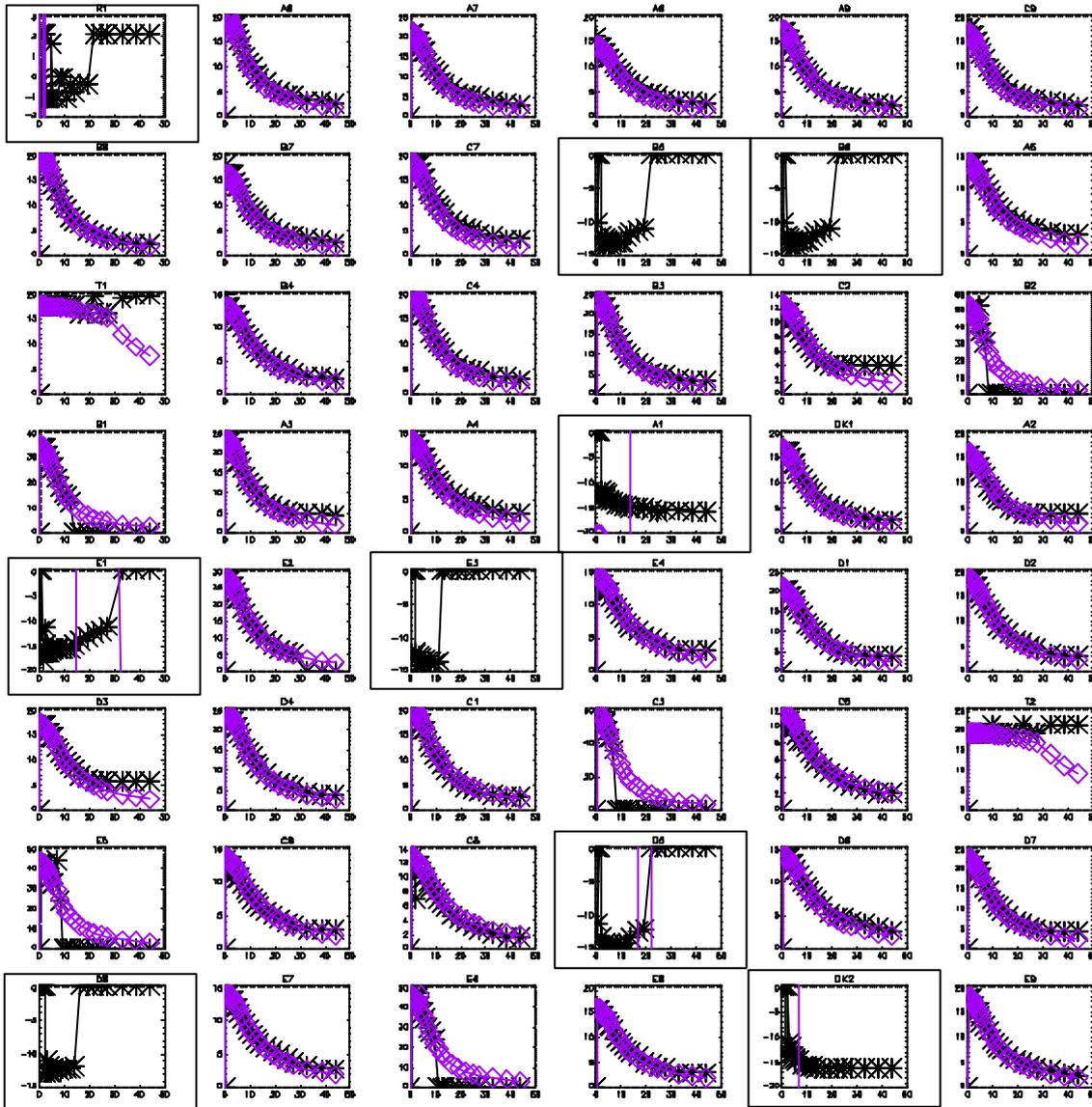
Figure 6: Derived  $R_{bol}$  as a function of bias voltage derived from phase change (black stars) and from the derived bias current and voltage across the bolometer (purple squares). This is for 130 Hz bias.
