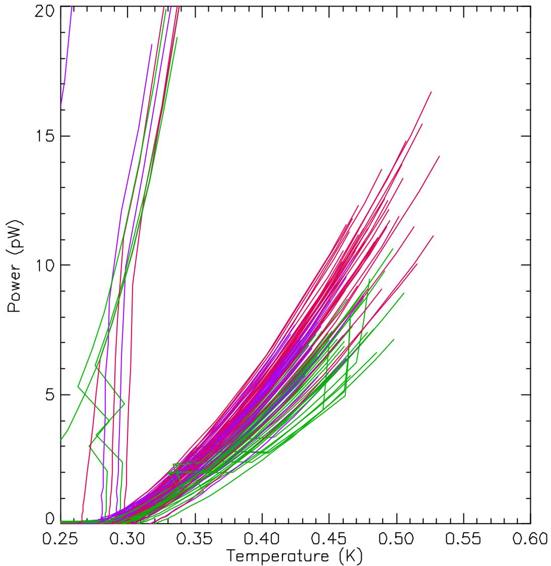
Figure 9: Corrected load curves for 70 (green); 130 (purple) and 190 (red) Hz plotted as Power versus temperature. Dead channels have been excluded – the vertical lines are for the resistor and thermistor channels. The strange lines in the 70 Hz data are where the offsets were mis-associated in the data.
