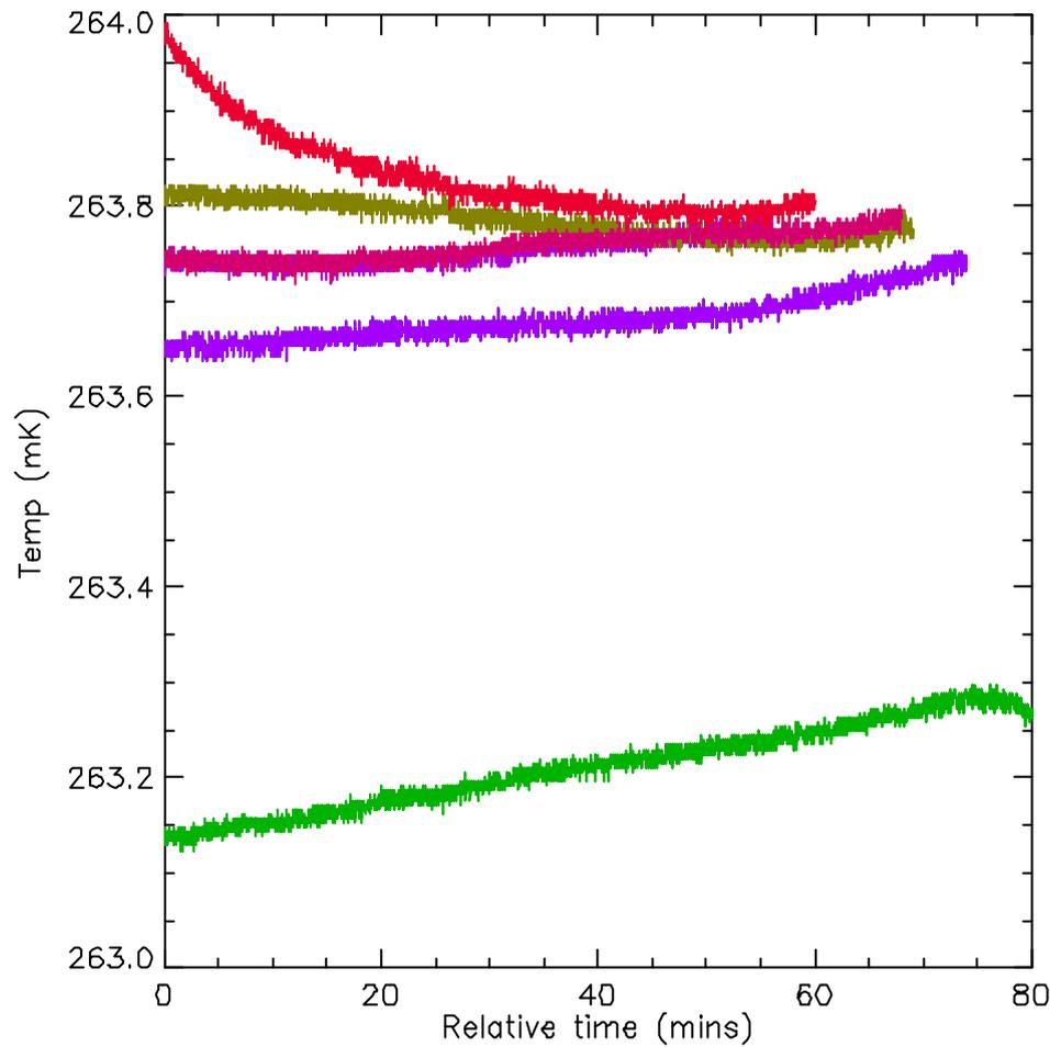
Figure 8: Evaporator temperature during the six loadcurves. Green(ish) is 70 Hz; Red(ish) 130 Hz and Purple (ish) 190 Hz. The brighter colour in each case is the in phase curve. The bottom green curve is for the 70 Hz in phase case.
