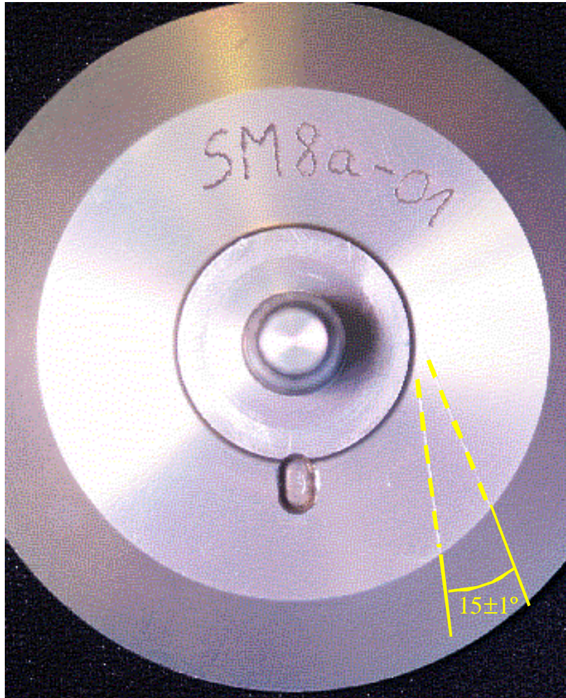
Figure 7. View of the back of SM8A showing marks made before and after rotation.
