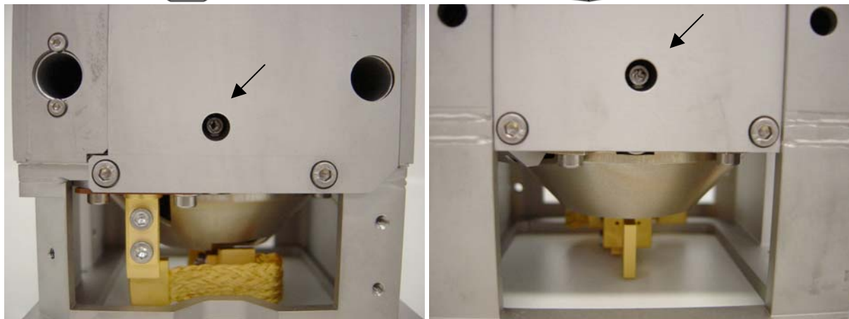
Centering screws – evaporator side
