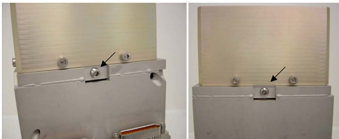
Centering screws – pump side
