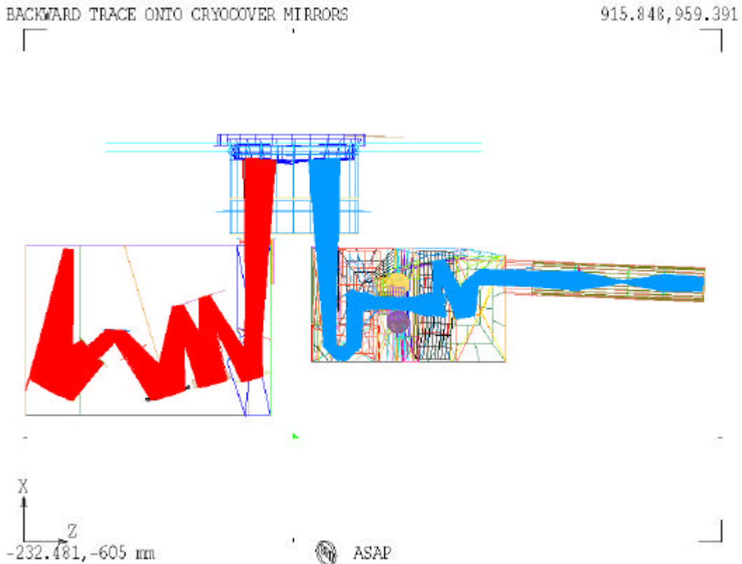
Figure 2.1-1: Configuration with two concave mirrors on the closed cryocover, backward trace of rays from the detectors onto the cryocover
