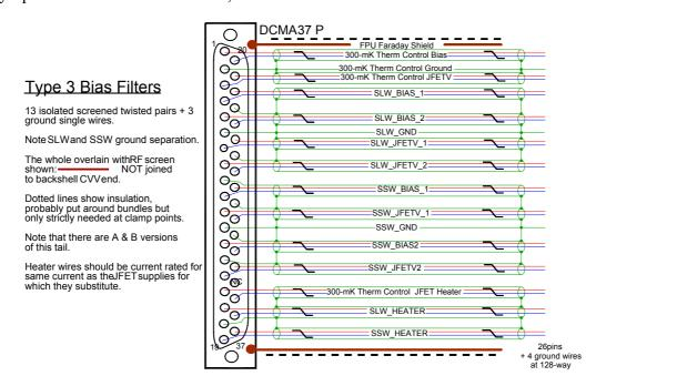
Because the small SLW has no subgroups that might fail, EACH of the JFET bachharness leads is double-wired in this cryoharness, requiring linked across in the filters.
