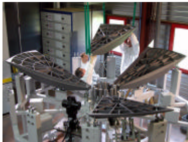
M1 in assembly for brazing
