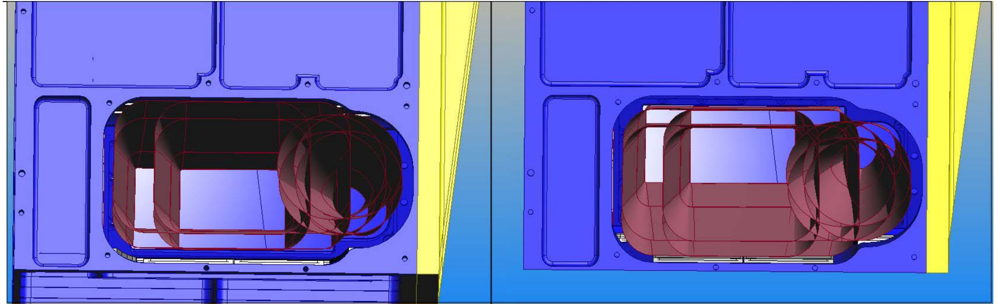
Figure 22 - Two views into SPIRE Input baffle showing clearance between the oversized beams and the tiles.
