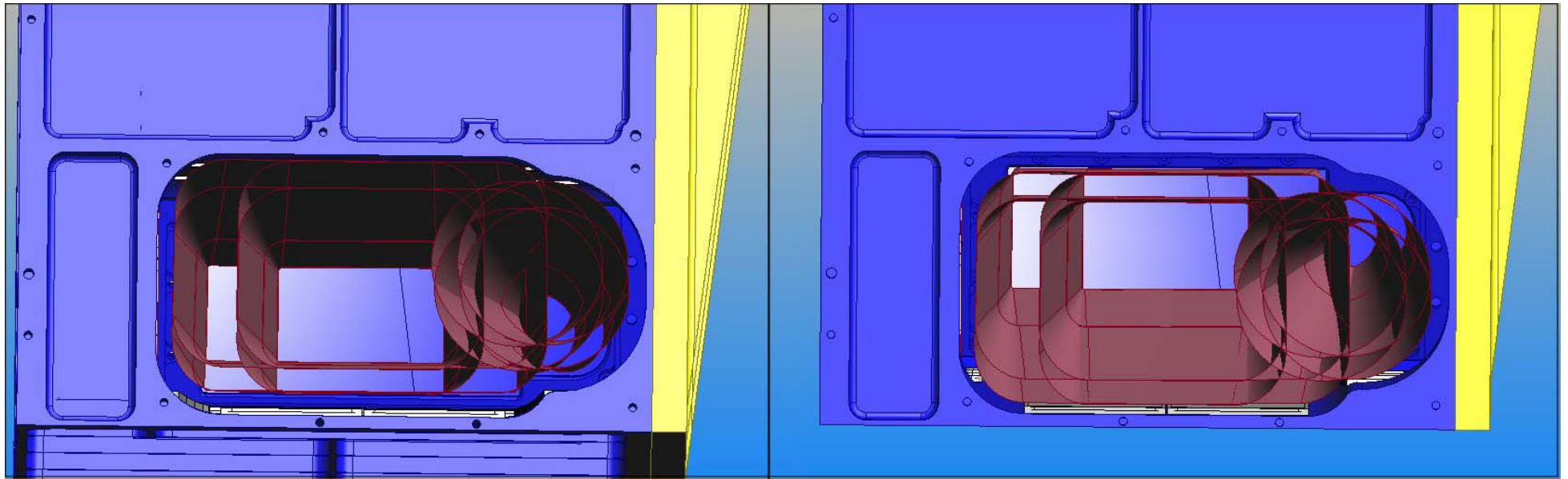
Figure 21 - Two views into SPIRE Input baffle showing clearance between the oversized beams and the tiles.
