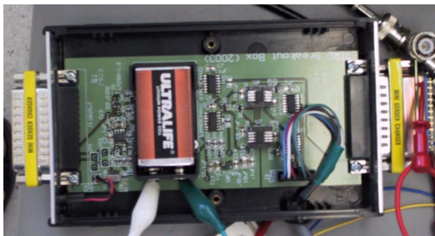
Figure 3: The break-out box
