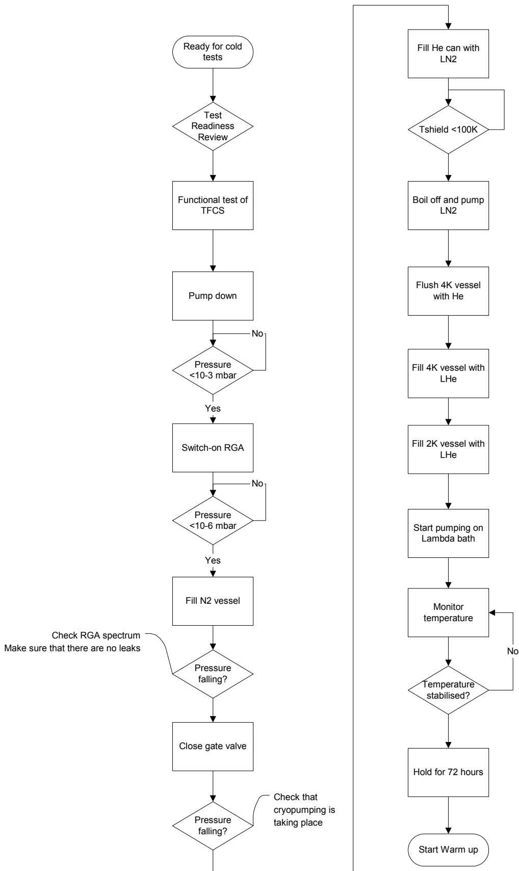
Figure 8: Flowchart showing sequence of activities for cold trials
