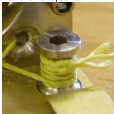
Figure 5 Details of Kevlar wrapping around fixed capstan at start of run.
