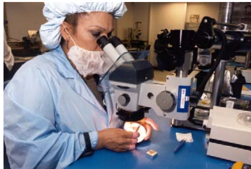
Component Attach- Bolometer/Load Resistor/ Flex Harness
