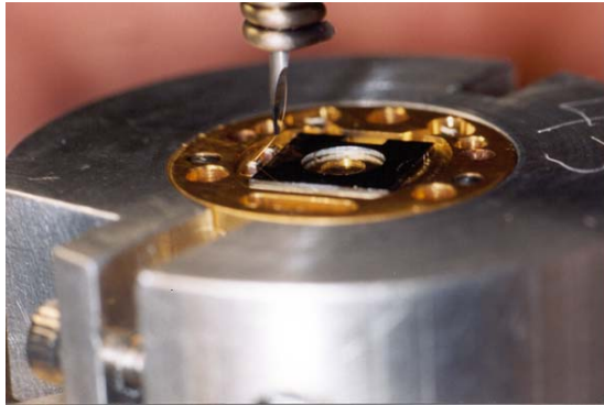
Wire Bonding- Bolometer/Load Resistor/Flex Harness
