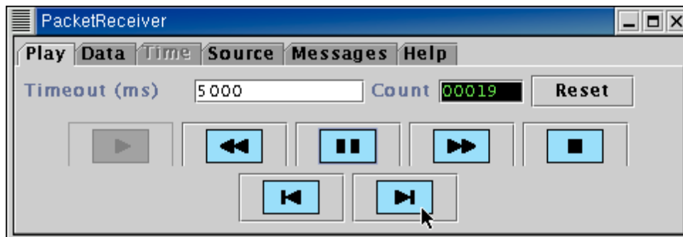
Figure 9: The PacketReceiver menu in playback mode, with the pause button having been pressed, and the step forward button being selected
