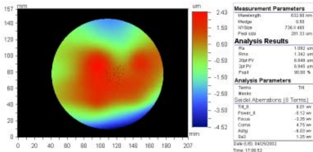
**Figure 5:** Contour plot of the reduced interferogram at the centre of F1. The analysis is performed on 90% of the max 150mm pupil aperture of the interferometer. The darkest red zones have been linked to the location of the M6 screws holding the tilt platform in the back of the mirror.
