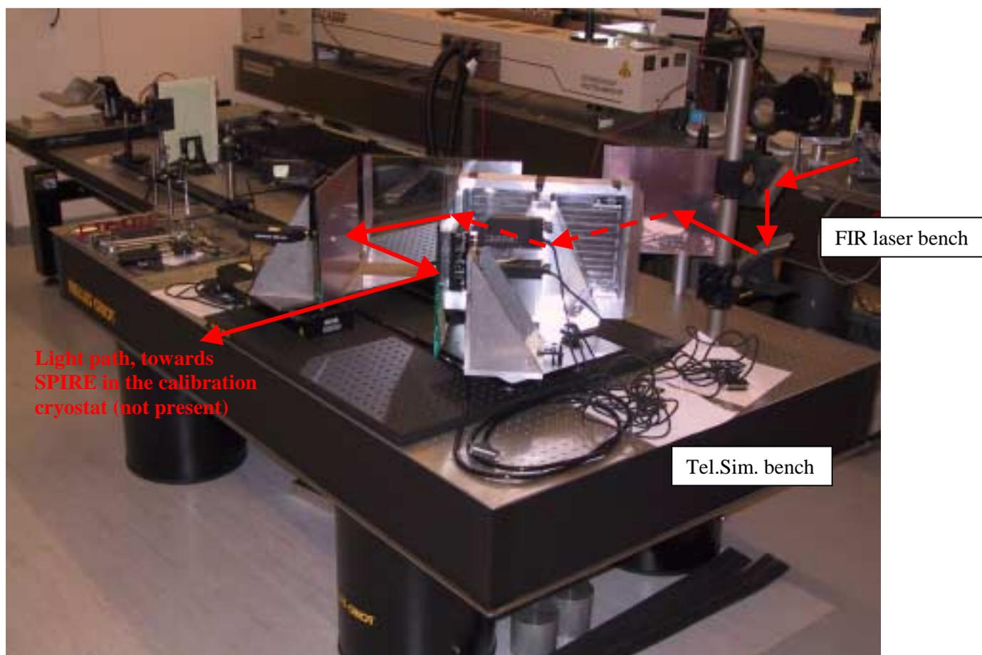
**Figure 1:** Telescope Simulator hardware in the SPIRE cryolab (03/05/2002)
