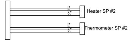
Each connector is interfaced with an electronic board which delivers the excitation current to heaters and thermometers and read in return the resulting voltage. These two electronic boards are totally segregated.
