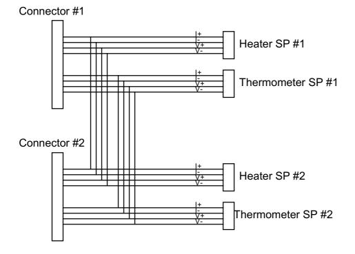
Then, each electronic board would be able to deliver the excitation current and to measure the temperature on both redounded heaters and thermometers of each component of the SCO, thus ensuring a higher fault tolerance and then a higher availability to the system. Effectively, in the preceding configuration, loss of heater #1 excitation and thermometer #2 excitation or measurement would lead to the mission loss when the proposed configuration would not.
