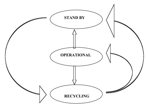
The modes transitions (by activating the heat switches) is driven by hot electronics (DRCU for SPIRE, BOLC for PACS). These drive electronics are identical for both instruments.
