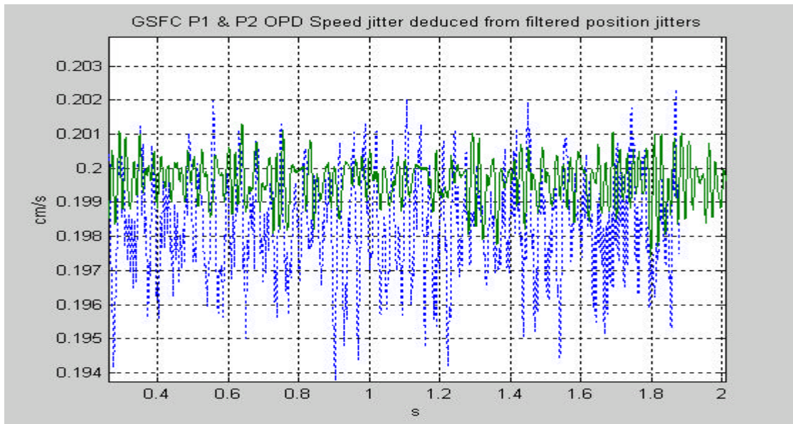
Figure 16 : OPD Velocity simulation for GSFC P1 & P2
