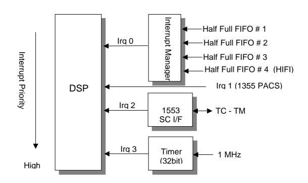
The task read from a preloaded table (exec\_matrix) the time to the next command and the command to transmit, it then set the timer and transmit the command to the SS. In order to avoid collision on the low speed I/F with the LS\_Task, a special (internal) command is foreseen to lock/unlock (via a mutex) the low speed I/F. The locking command will precede the SS commands of at least 100 us in order to allow the possible contemporary (just started) transmission of a command via the LS\_Task.
