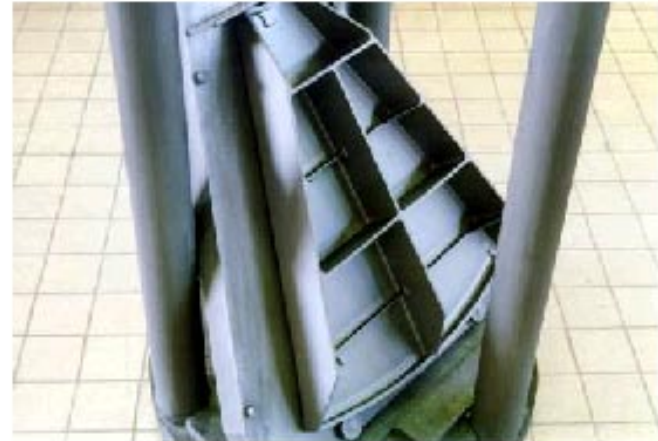
2- Segment sintering (Boostec)
