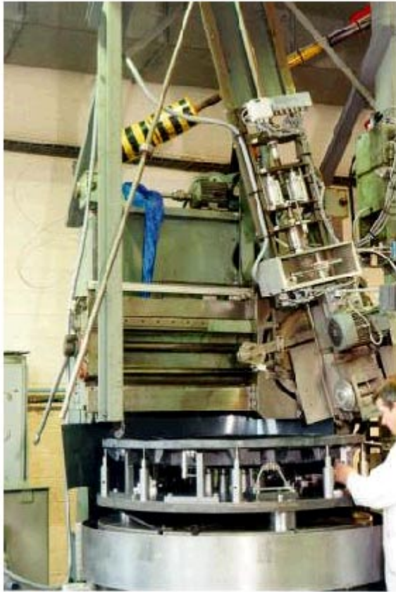
5- Grinding of optical face (Boostec)
