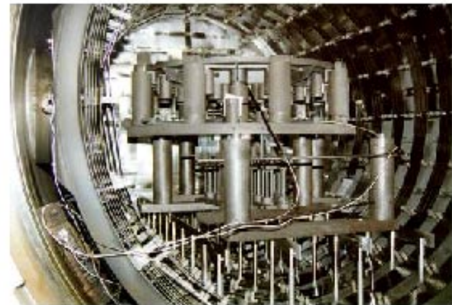
4- Brazing (Boostec + Astrium support) IABG oven TBC
