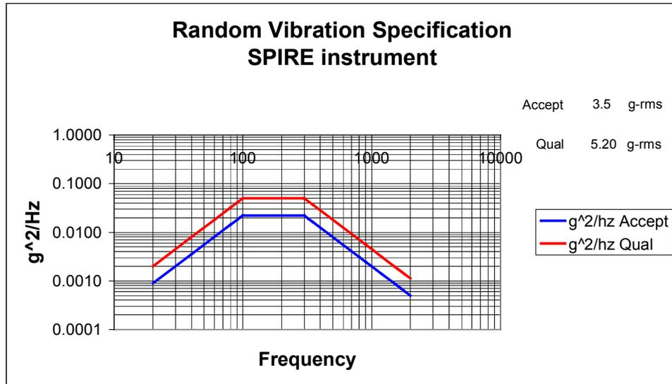
Figure 2: Random spectrum definition for all 3 directions (x, y and z)
