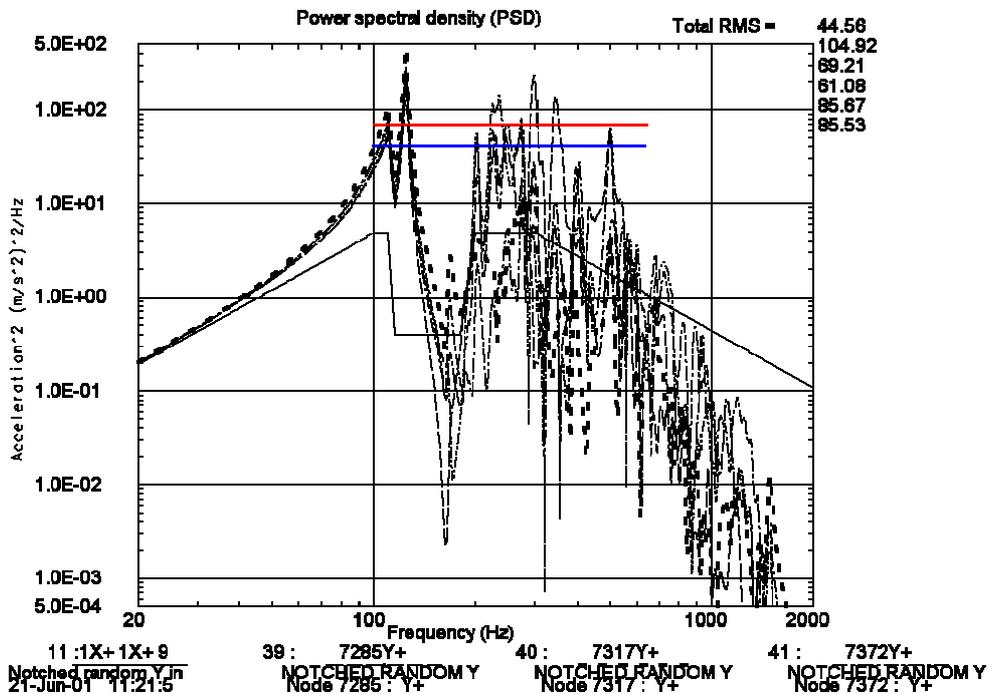
Figure 4: Response at the base of the BDA due to notched input given in the same figure (solid black line)
