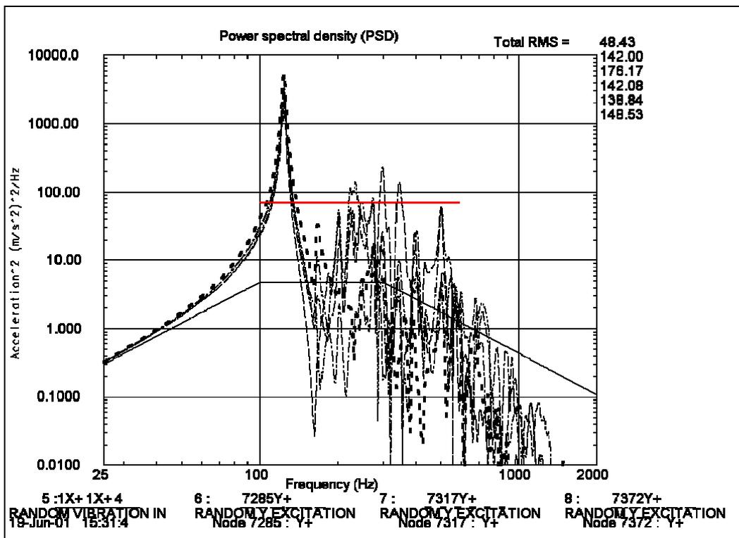
Figure 3: Response at the base of the BDA due to un-notched input given in figure 2
