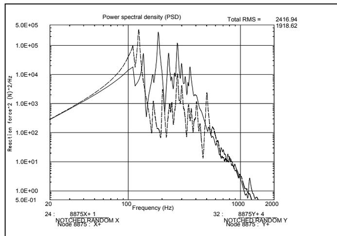
Figure A-3: Notched X and Y -input X=2.4 kN Y=1.9 kN (rms)
