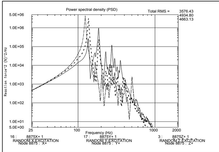
Figure A-1: Un-notched I/F force for the three orthogonal directions
