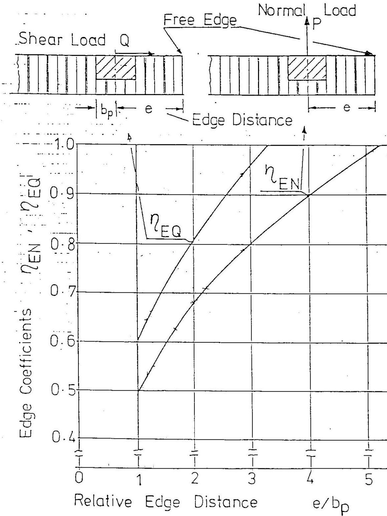
Figure 4.7-2: Influence of edge distance on the static strength capability of inserts
