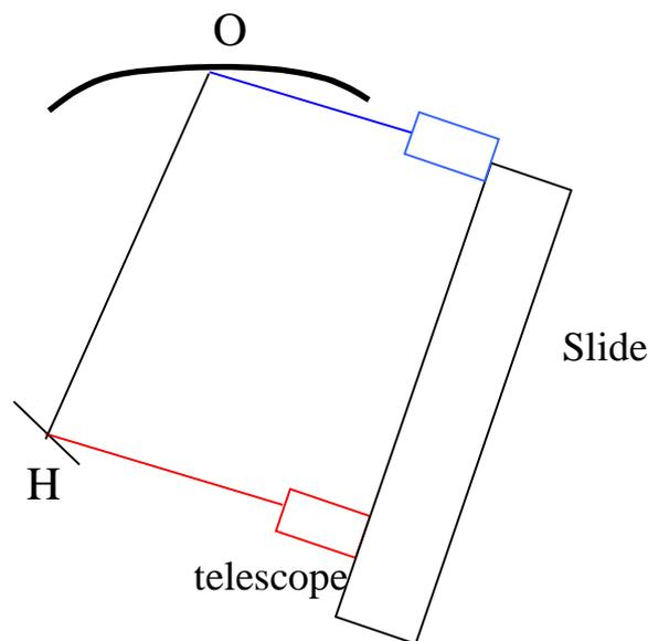
Using a fixed focus for the AT ensures that the OH is parallel to the slide direction. The slide mounting should ensure that the slide travel is horizontal, i.e. parallel to the bench, so that OH is too (for in-plane propagation). The distance OH is set to the  $R_{SM}$  value (see RD1 and RD2 for details concerning constraints and consequences of this value).
