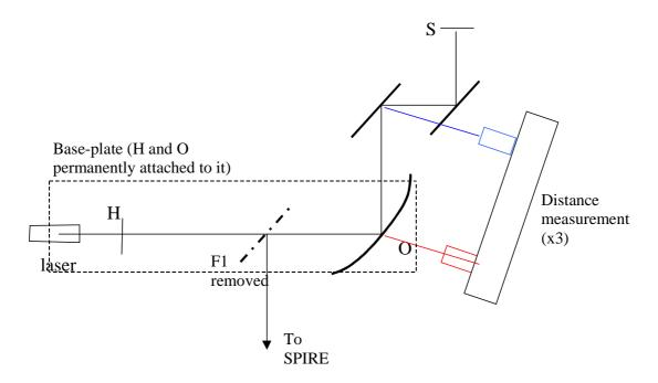
The angular position of S is given readily by the trace laser beam from H (the fold mirror F1 has to be removed to see it). The linear position along the focus direction is more difficult to set, because visible imaging can't be made, and it is hard to measure the fold path length accurately.
