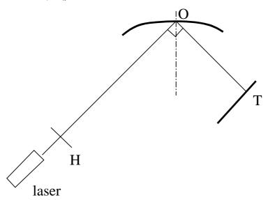
In general, angle-alignment at O will lead to linear-position drift, and this must be monitored & corrected during alignment i.e. the position & angle at O must be iterated until both are within spec. Because the mirror is large, shims will be used and need to (re-)calculated at each iteration.
