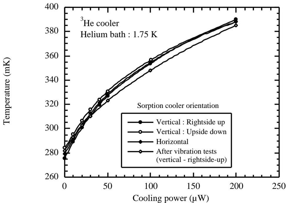
*<sup>3</sup>He Sorption cooler – cooling power curve*
