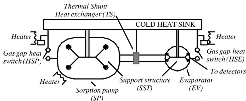
As shown on the above figure, a helium sorption cooler is basically made of 6 components designated as a sorption pump SP and an evaporator EV connected via a pumping line to a thermal shunt TS comprising an heat exchanger, two gas gap heat switches HSP and HSE respectively connected to the sorption pump (SP) and evaporator (EV), and
