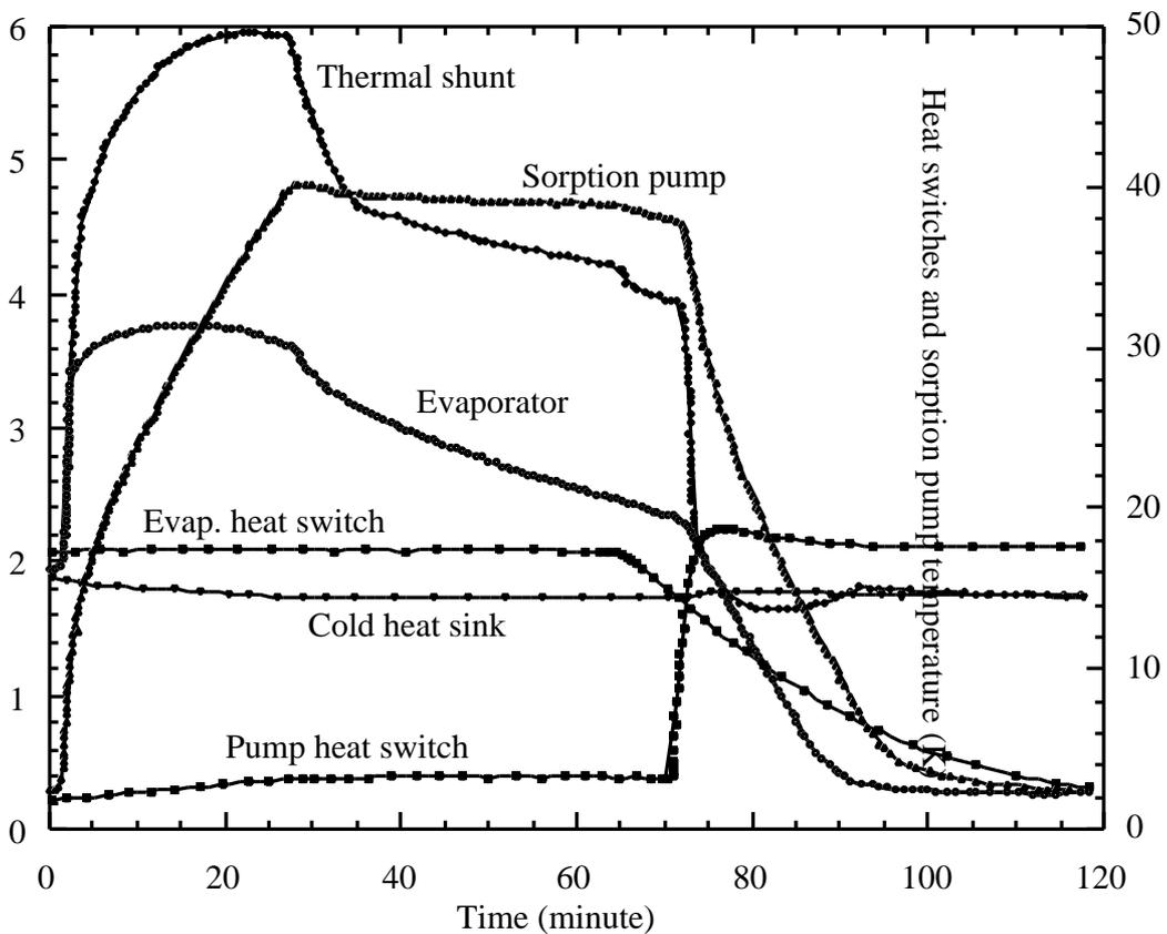
Evaporator, shunt and cold plate temperature (K)
