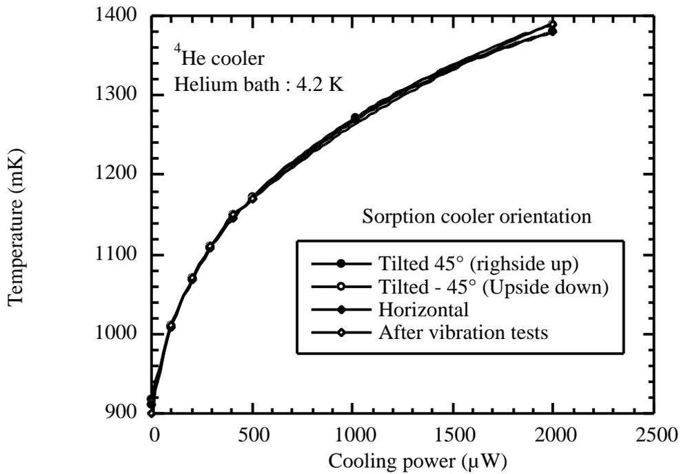
*<sup>4</sup>He Sorption cooler – cooling power curve*
