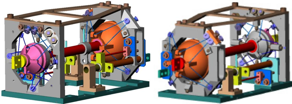
*$^3\text{He}$  cooler Evaporator (top) and sorption pump side*
