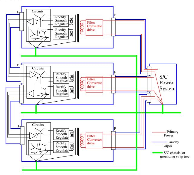
Each unit is electrically self-contained in its grounding.
