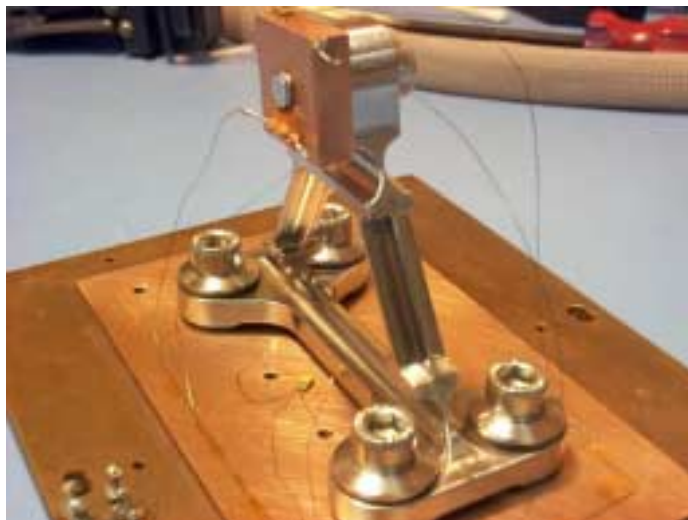
Figure 4-41 - FPU/HOB interface strut.
