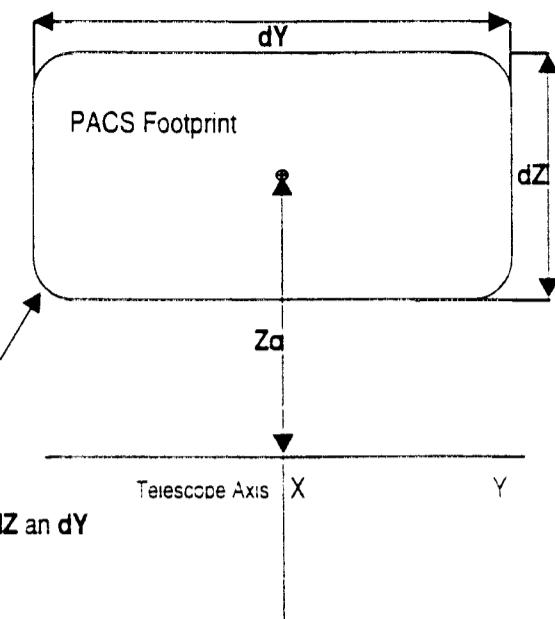
After finding the net beam geometry we then need to add 20 mm (10 mm radial "zone of avoidance") to quantities  $dZ$  and  $dY$  to allow for diffraction and alignment margins.
