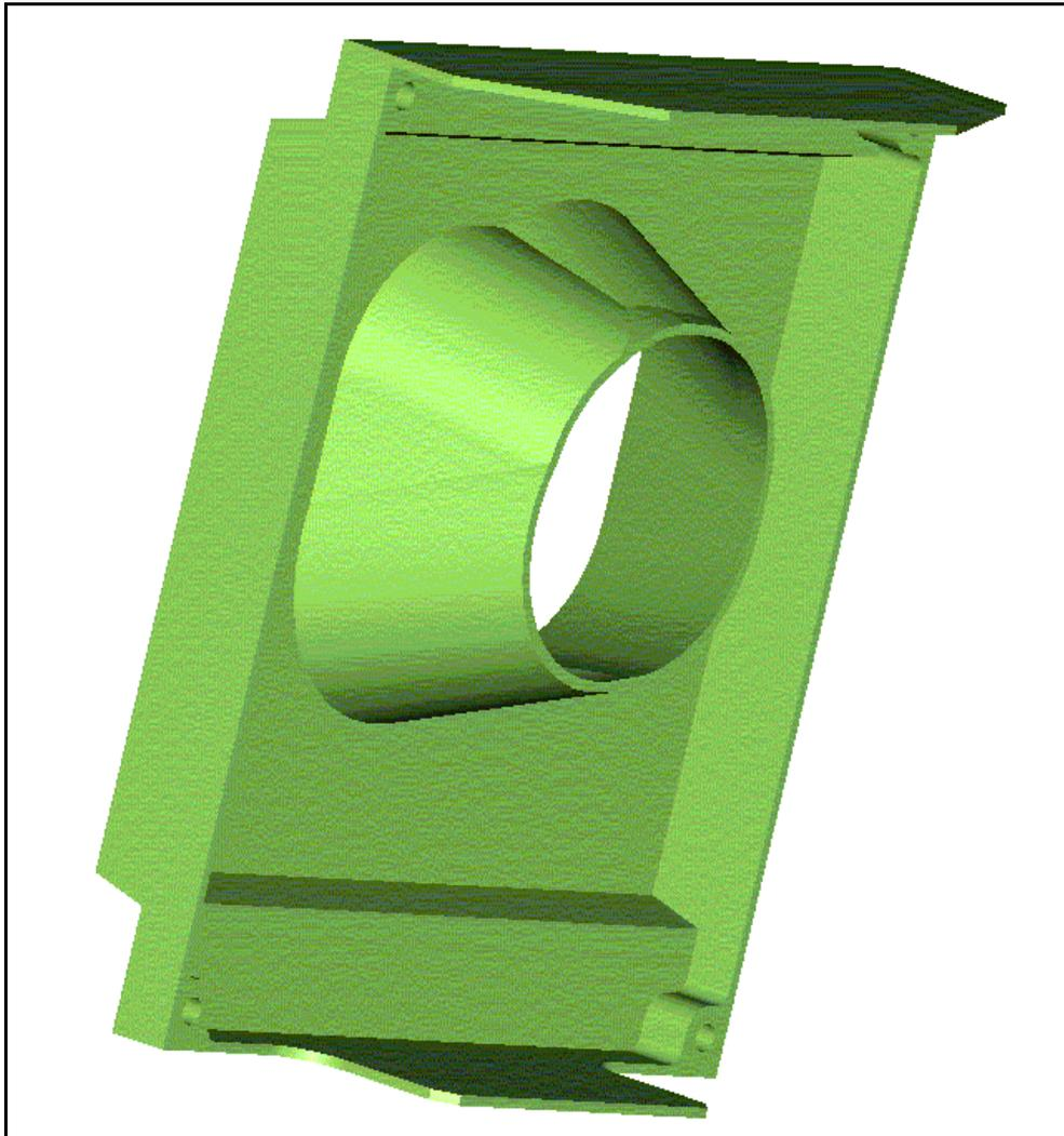
Figure 23: BSM baffle concept: general plate thickness 1mm The baseline design would be the same as this but have no 'cone'.
