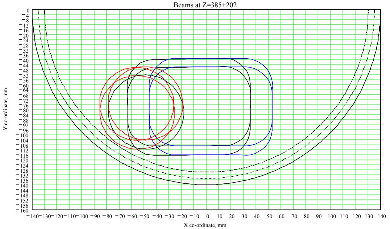
**Figure 4-3 Composite beam boundaries at 385 mm forwards of the telescope axial focus**
