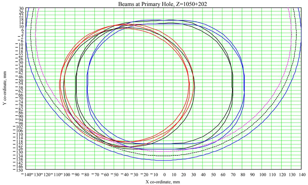
**Figure 4-1 Composite beam boundaries at 1050 mm forwards of the telescope axial focus**
