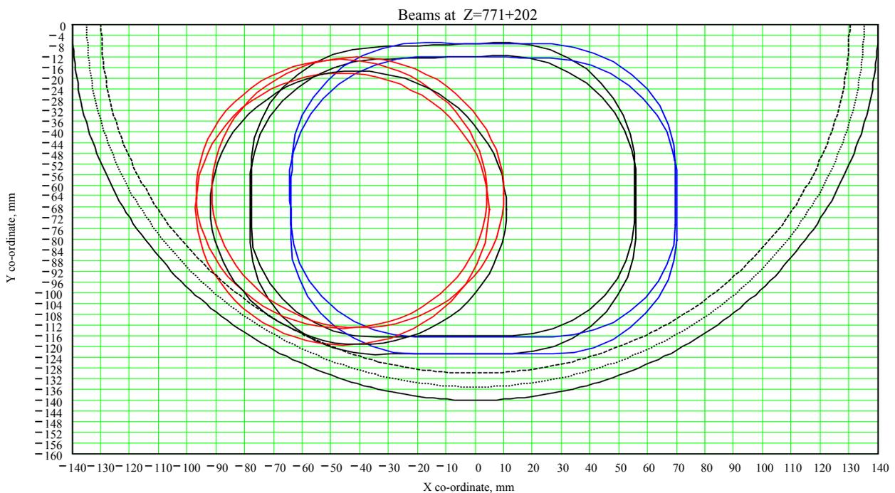
**Figure 4-2 Composite beam boundaries at 771 mm forwards of the telescope axial focus**
