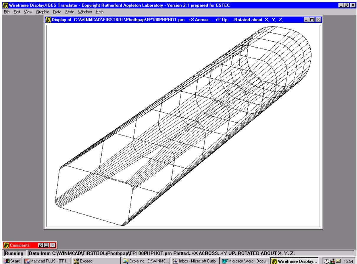
**Figure 3-2 Wire-frame representation of a composite photometer beam boundary**
