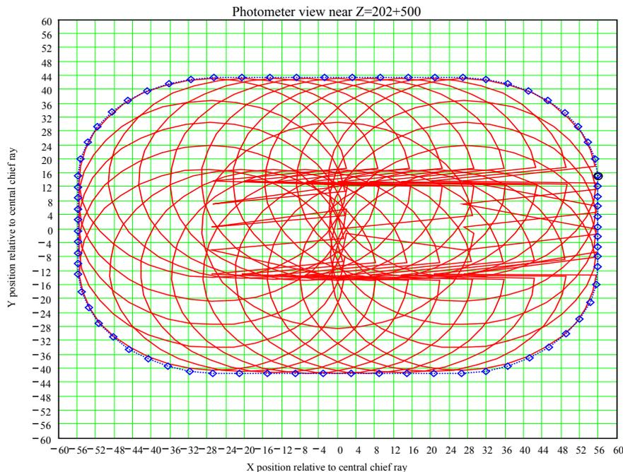
**Figure 3-1 Photometer beam envelope 500 mm forwards of telescope focal surface**
