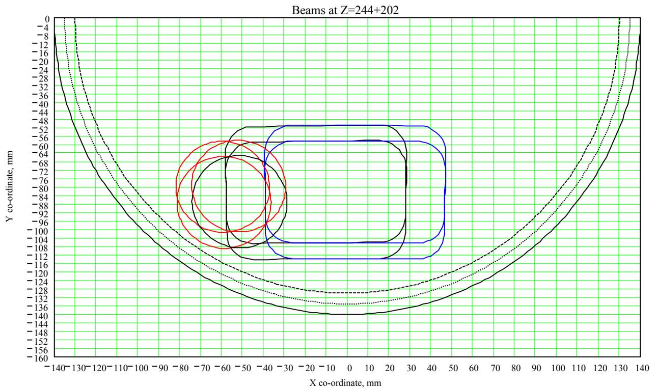
**Figure 4-4 Composite beam boundaries at 244 mm forwards of the telescope axial focus**
