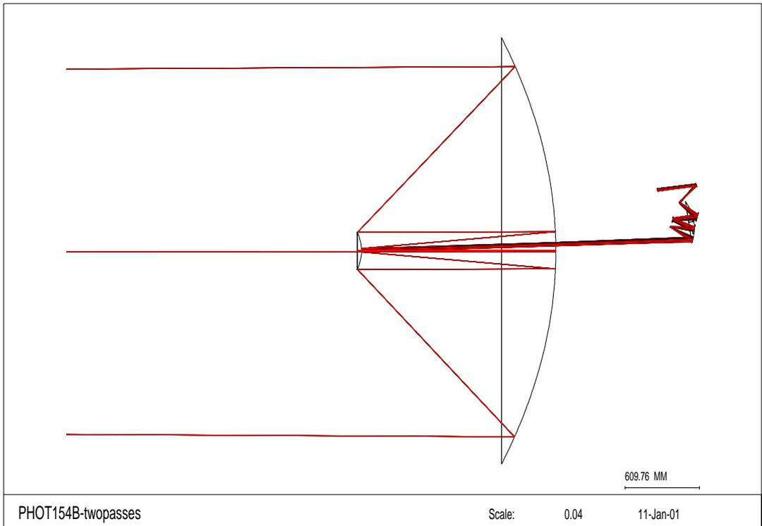
**Figure 6 Rays converging on detector image at 290 metres after two passes through the telescope**
