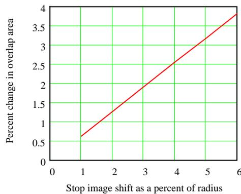
**Figure 13 Percentage throughput loss as stop image is shifted**
