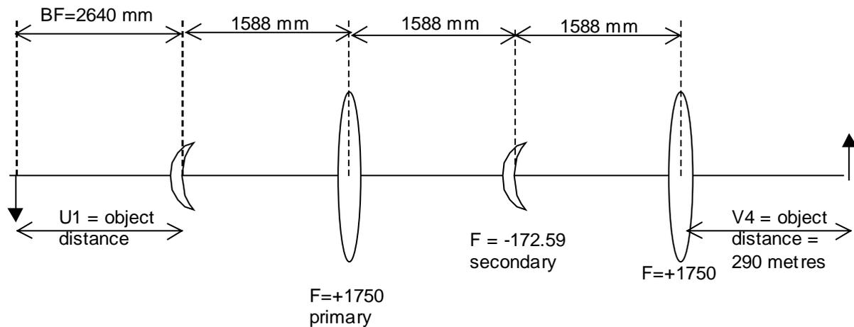
Mirrors are represented as lenses with focal lengths = 1/2 the radius of curvature at the pole
