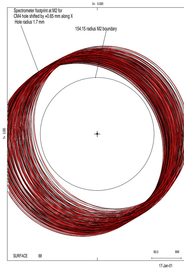
**Figure 10 Composite footprint of spectrometer beams at M2, defined by a 1.7-mm radius stop at CM4 shifted by +0.65 mm along X**
