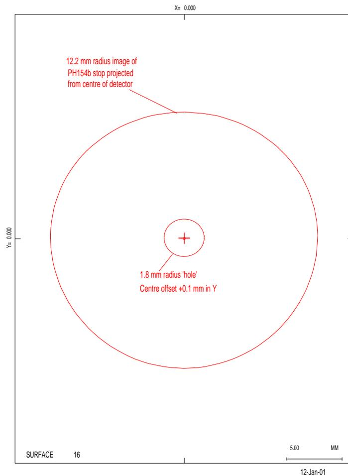
**Figure 11 Proposed 'hole' in CM4 compared to total photometer beam area**
