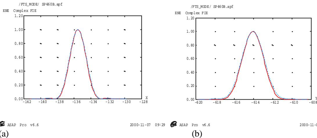
Fig.4. Far-field beam pattern for cases without focus compensation (solid line) and with (dotted line). (a) in x-section (b) in y-section.
