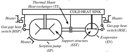
Cryogenic switches can be based upon different physical mechanisms. Gas gap heat switches have been selected as the preferred design for the present project. Gas gap heat switch utilizes concentric copper cylinders separated by a small gap which is filled with or emptied of He gas to achieve the switching action. The thermal separation between the two ends is achieved by a thin-walled tube which also provides the mechanical
