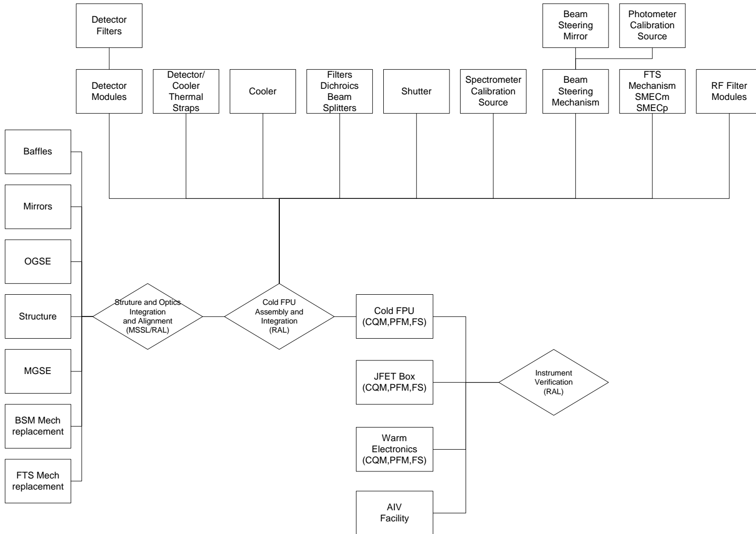
Figure 3-5: Deliverable sub-systems for the SPIRE Instrument level AIV for all cold FPU models
