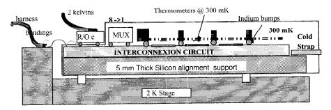
The read out circuit must be at 2 K, but close to the IC to control and minimise the electrical capacity and then the signal bandpass.
