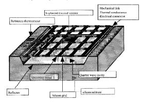
response through arrays (flat spatial response) easy multiplexing and power dissipation at cold stage a very high impedance for sensors was chosen (10-100  $G\Omega$ ).
