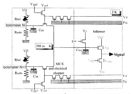
The measured thermal sensitivity (1.5  $\mu$ K/ÅHz) of the thermometers imposes a large thermal impedance between the bolometer and the silicon substrate to achieve the desired NEP. The thermal bandpass is then limited to 15 -20 Hz.
